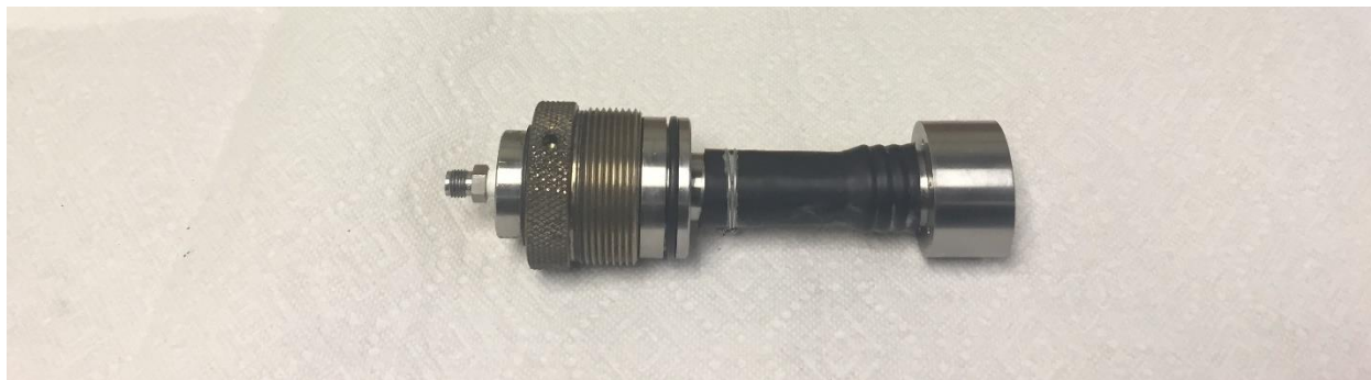
Figure A.3: Core plug in black polyolefin jacketing attached to flow distributors
