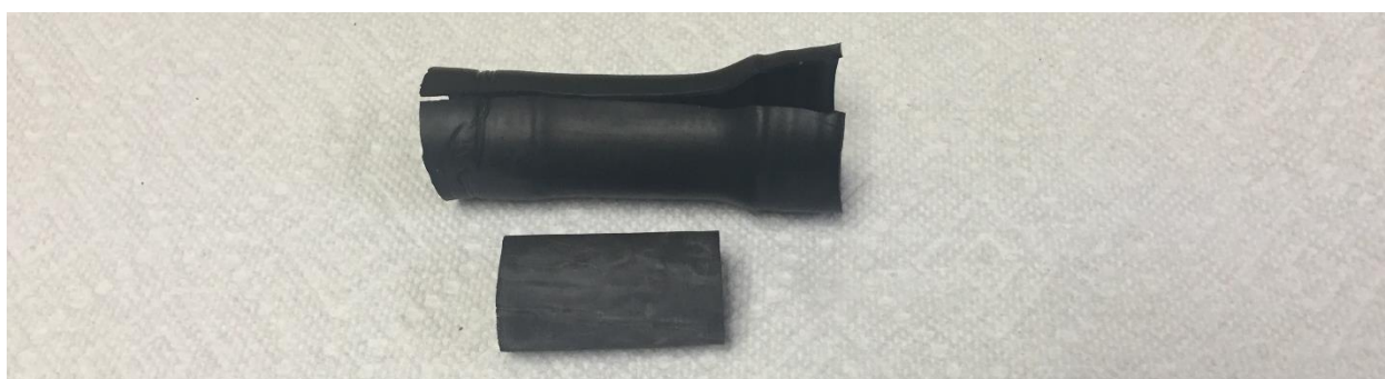
Figure A.4: Core plug sample extracted from jacketing at the end of an experiment
