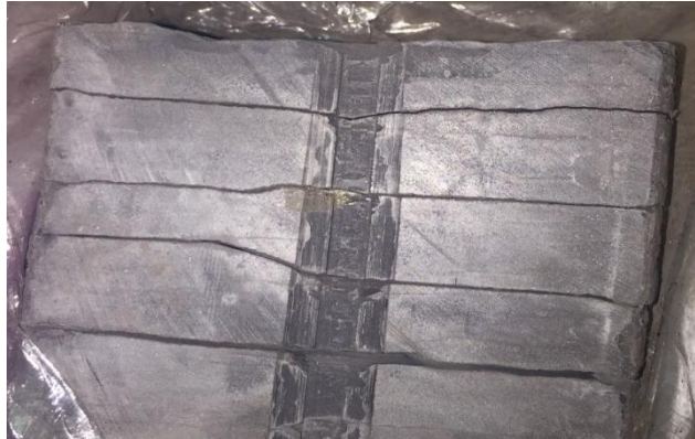
Figure 3.2: Slabbed Marcellus core - 3.8cm (1.5") diameter and 3cm in length showing multiple parallel to lamination fractures spaced 2-3cm apart
