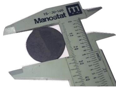
Figure 3.6: 2mm length Marcellus sample used for single phase brine permeability measurement at steady state flow conditions
