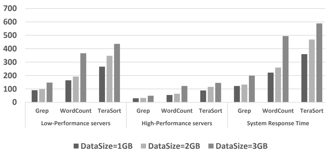
Figure 6-2. The MST of heterogeneous nodes with the fair job scheduler.
