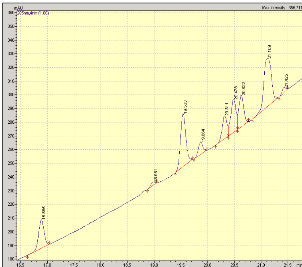
Figure 3-7. Chromatogram for the combined standard (wavelength= 205 nm) analyzed using an RP-Amide stationary phase and methanol (MeOH) mobile phase.
