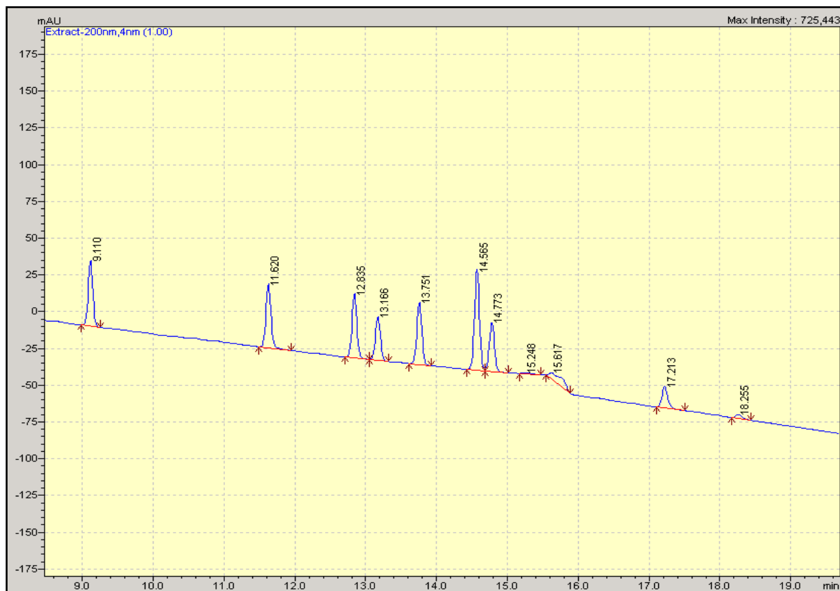
Figure 3-4. Chromatogram for the combined standard (wavelength= 200 nm) analyzed using a Biphenyl stationary phase and acetonitrile (ACN) mobile phase.
