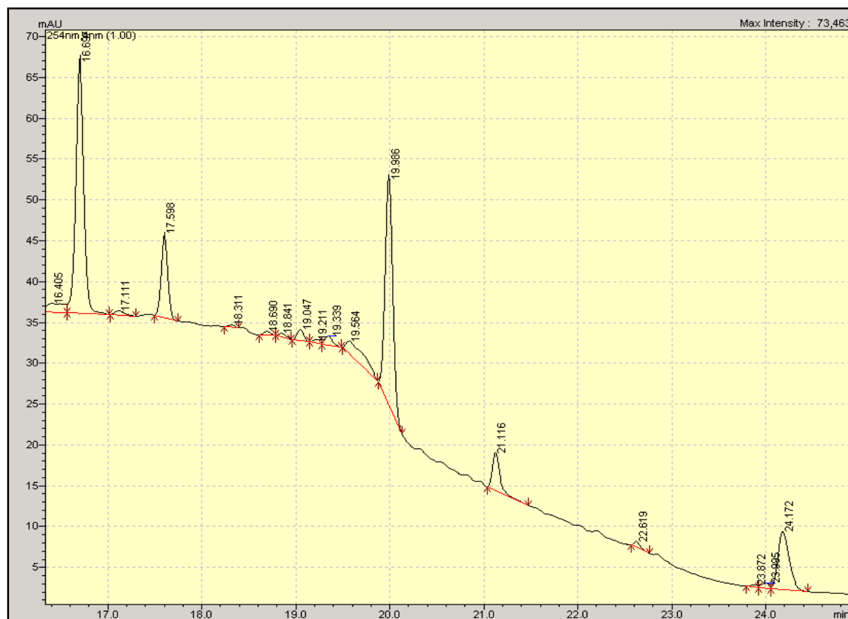
Figure 3-10. Chromatogram for the combined standard (wavelength= 254 nm) analyzed using a Biphenyl stationary phase and methanol (MeOH) mobile phase. The peaks at 16.7, 20.0, and 24.2 minutes are genistein, biochanin A, and progesterone respectively.
