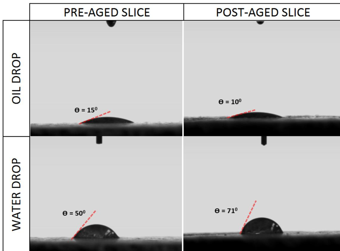
Figure 5-1: Oil and water drop images captured by the Drop Shape Analyzer during contact angle measurement on pre-aged and post-aged core slices.
