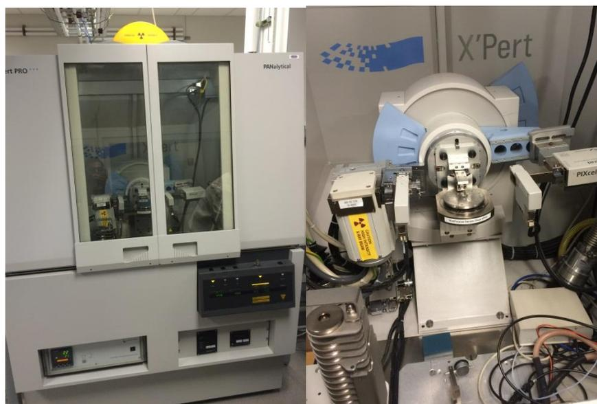
**Figure 4-3: Outside of Diffractometer (left) and Inside of Diffractometer (right)**
