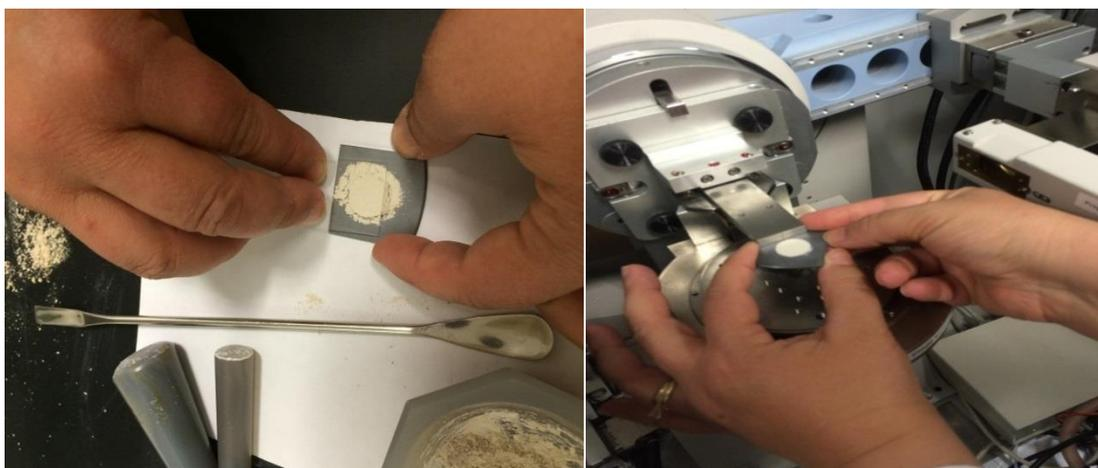
**Figure 4-2: Powdering the rock (left) and placing it in the X-Ray Diffractometer (right)**
