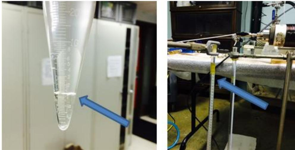
**Figure 4-11: Flow Collectors for Oil Injection (left) and Waterflooding (right). Sensitivity of the tube used during oil injection was  $\pm 0.05$  cc while it was  $\pm 0.1$  cc during waterflooding.**
