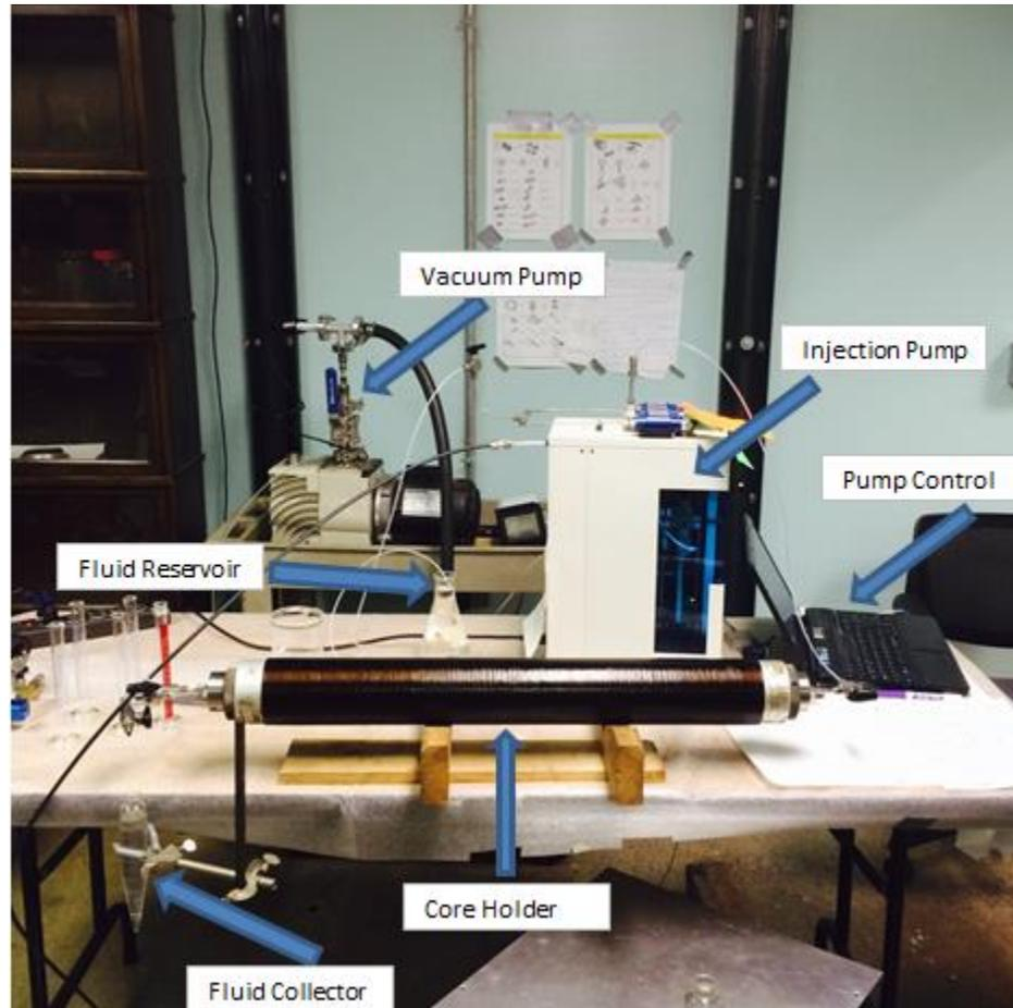
**Figure 4-8: Experimental Set-up for Waterflooding**
