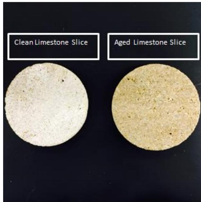
**Figure 4-13: Core Slices Used for Contact Angle Measurement**
