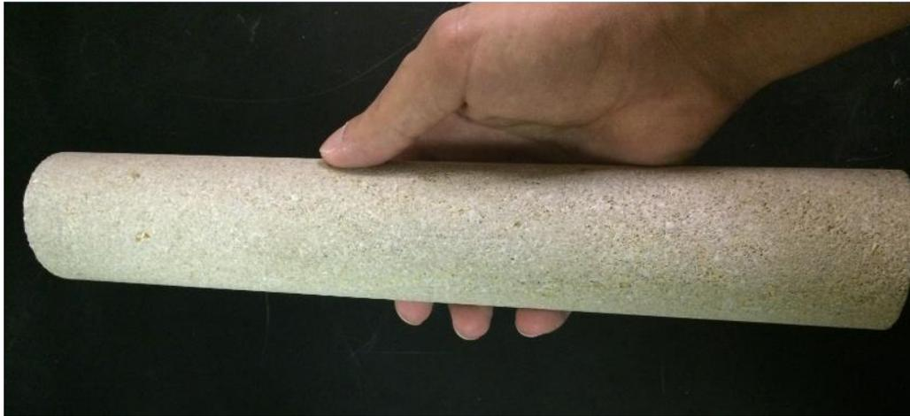
**Figure 4-1: Indiana Limestone Outcrop Cores used in Experiments**
