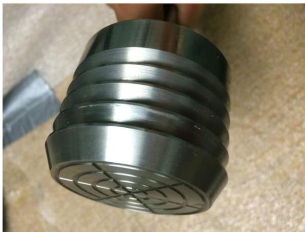
**Figure 4-10: Flow Distributor Built by EMS Machine Shop @ The Pennsylvania State University**
