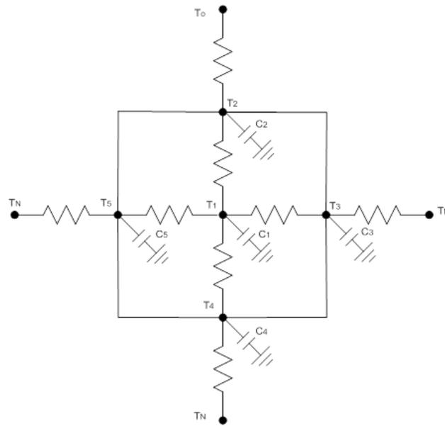
Figure 3.1. Single room thermal network model.
