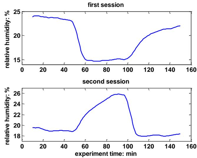
Figure 2.3. Measured relative humidity (RH) during the experiment.
