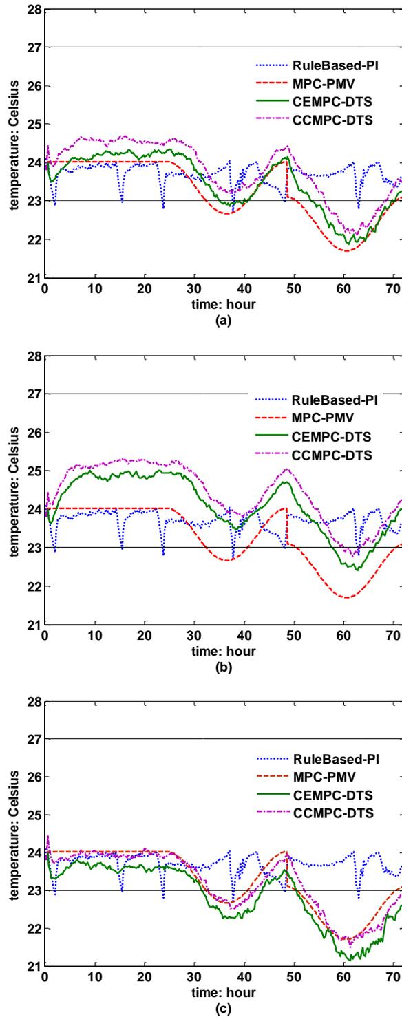
Figure 3.5. Controlled indoor air temperature. (a) Scenario I (March,  $E[w]=0$ ). (b) Scenario II (March,  $E[w]=-0.2$ ). (c) Scenario III (March,  $E[w]=0.2$ ).
