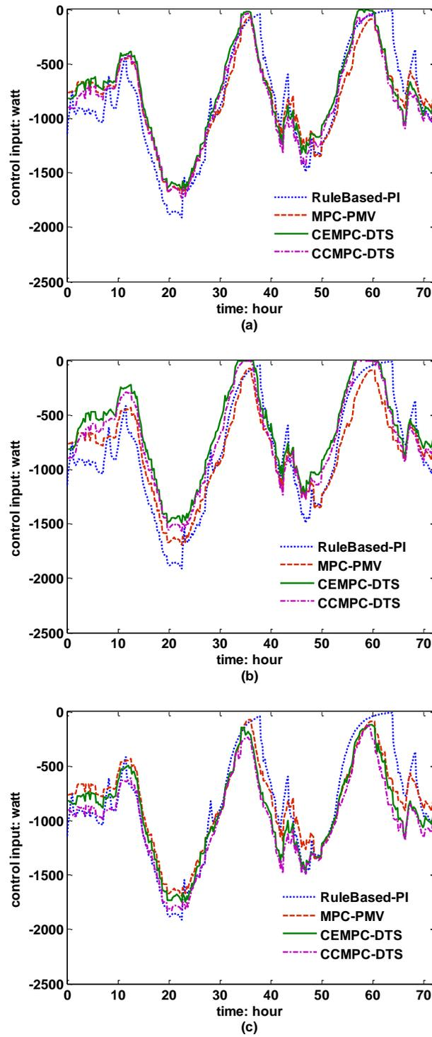
Figure 3.8. Control input. (a) Scenario IV (September,  $E[w]=0$ ). (b) Scenario V (September,  $E[w]=-0.2$ ). (c) Scenario VI (September,  $E[w]=0.2$ ).
