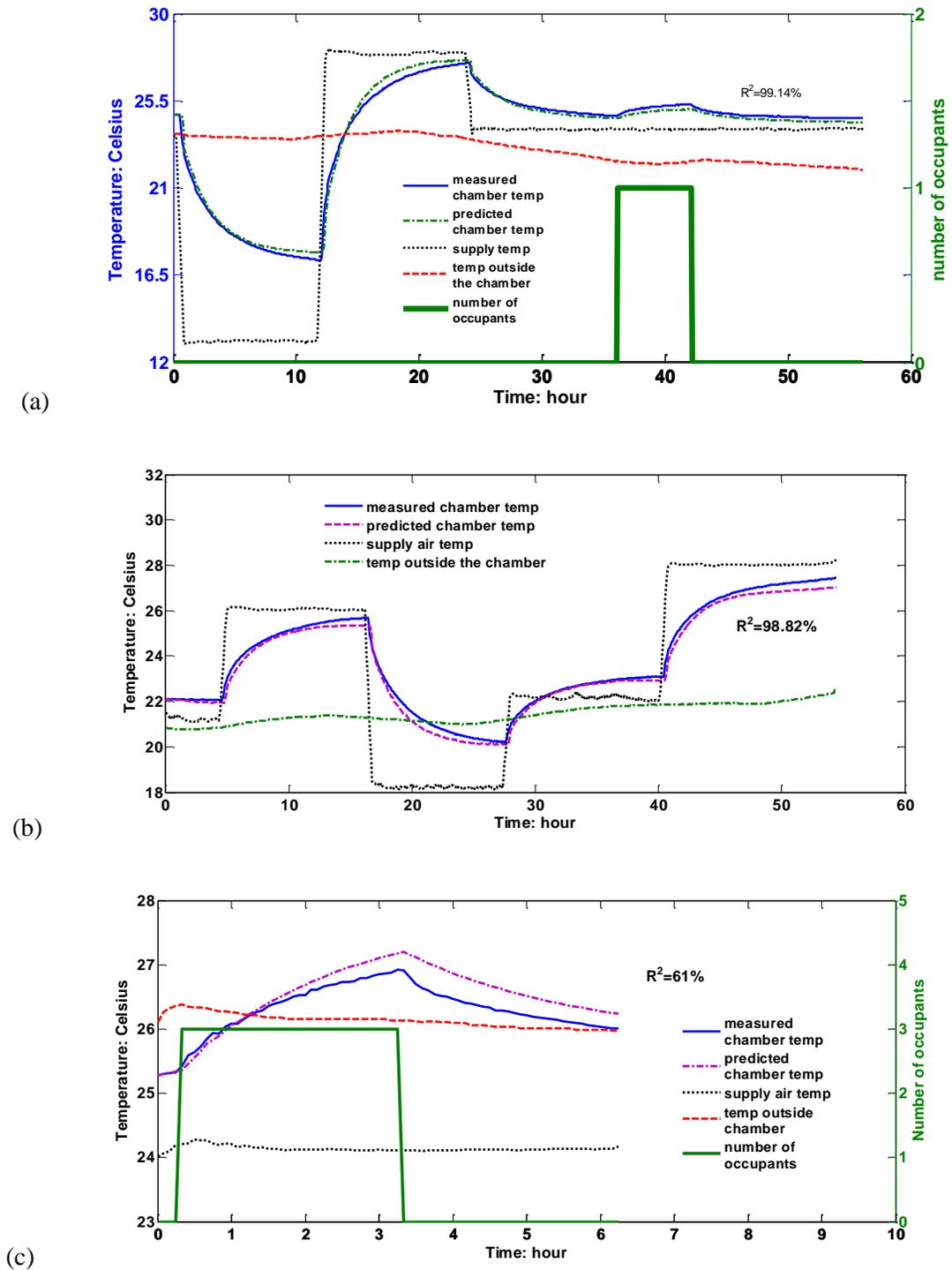
Figure 4.3. Chamber model identification and model validation. (a) predicted chamber temperature vs. measured chamber temperature under the training supply air temperature,  $R^2 = 99.14\%$ ; (b) model validation using a new trajectory of supply air temperature with no occupant,  $R^2 = 98.82\%$ ; (c) model validation using a new trajectory of number of occupants,  $R^2 = 61\%$ .
