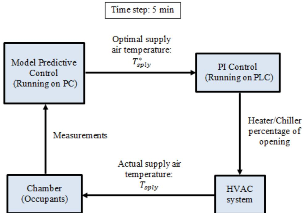
Figure 4.4. Diagram of a two-level control. On the top level, a MPC running on a PC determines the optimal supply air temperature; on the low level, a PI control running on PLC regulates the Heater/Chiller percentage of opening of the HVAC system to achieve the optimal supply air temperature. For the MPC-DTS, the MPC receives measurements of occupants (votes on thermal sensation) and for the MPC-PMV, the MPC receives measurements of chamber thermal conditions to compute PMV.
