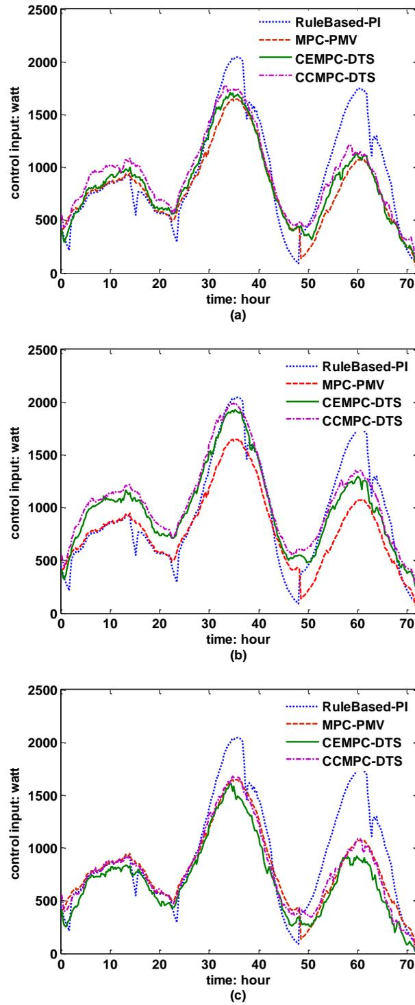
Figure 3.7. Control input. (a) Scenario I (March,  $E[w]=0$ ). (b) Scenario II (March,  $E[w]=-0.2$ ). (c) Scenario III (March,  $E[w]=0.2$ ).
