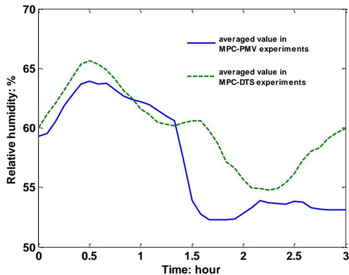
Figure 4.5. Mean history of chamber air relative humidity.
