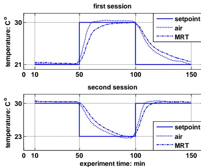
Figure 2.2. Measured and set point air temperatures and mean radiant temperatures (MRT) during the experiment.
