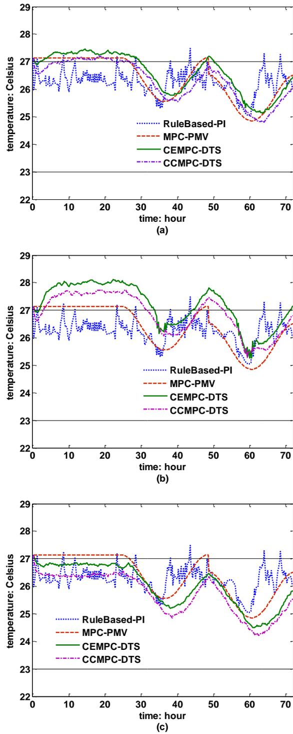
Figure 3.6. Controlled indoor air temperature. (a) Scenario IV (September,  $E[w] = 0$ ). (b) Scenario V (September,  $E[w] = -0.2$ ). (c) Scenario VI (September,  $E[w] = 0.2$ ).
