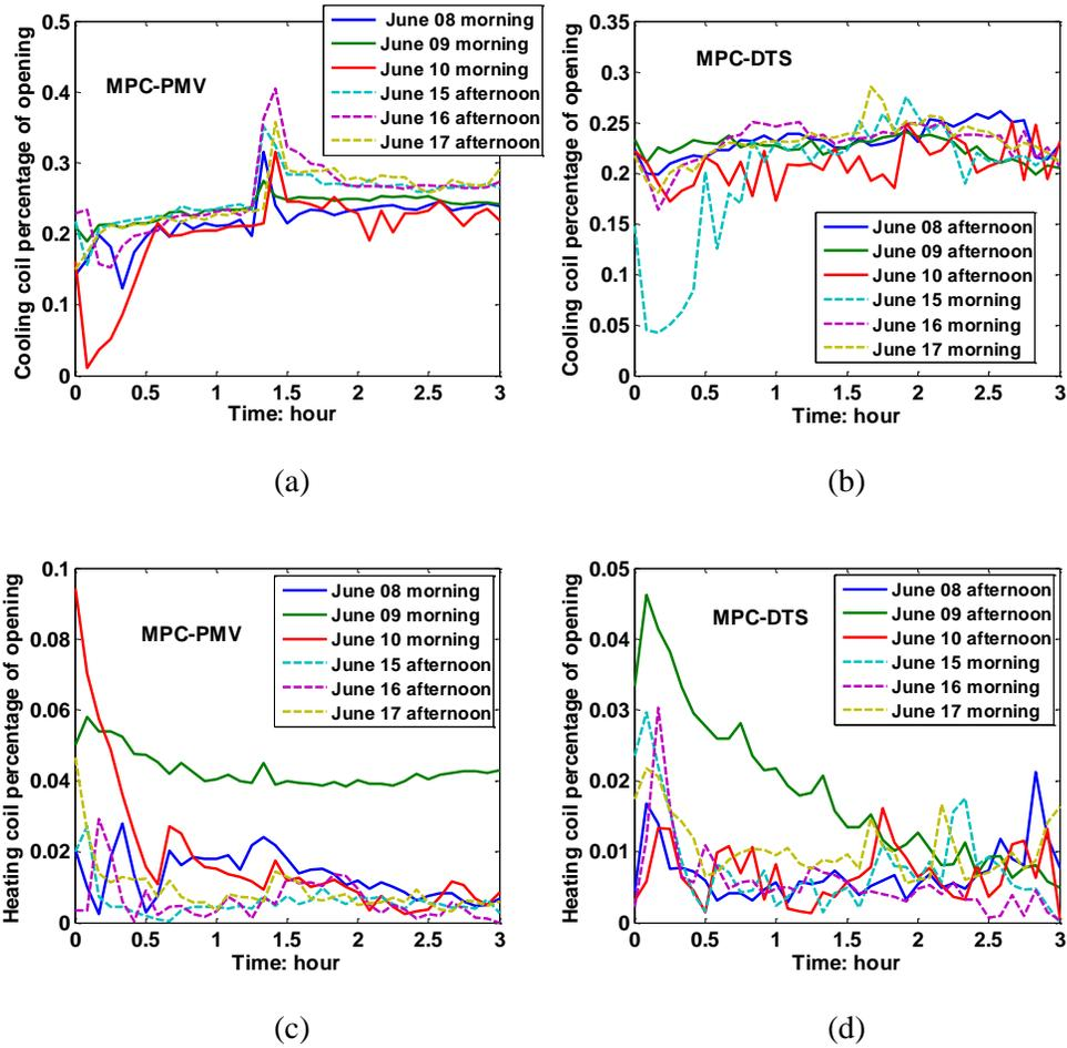
Figure D.5. Heating/Cooling coil percentage of opening. (a) Cooling under MPC-PMV. (b) Cooling under MPC-DTS. (c) Heating under MPC-PMV. (d) Heating under MPC-DTS.
