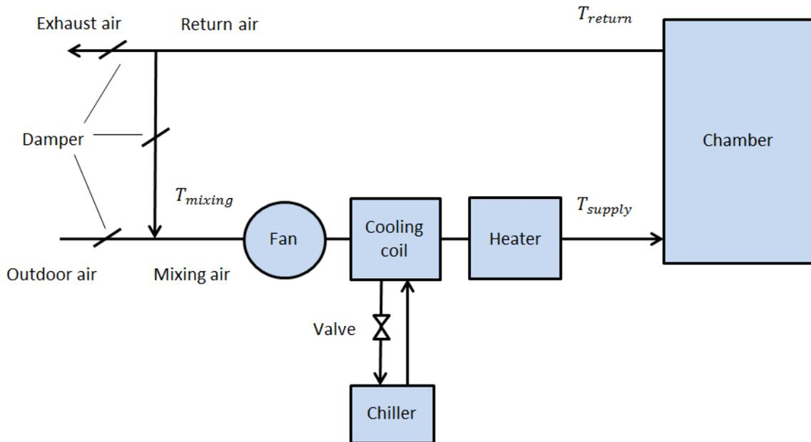
Figure 4.2. Chamber HVAC system schematic drawing.
