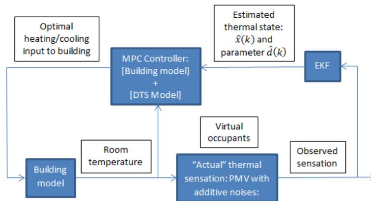
Figure 3.2. Block diagram for DTS model based MPC.
