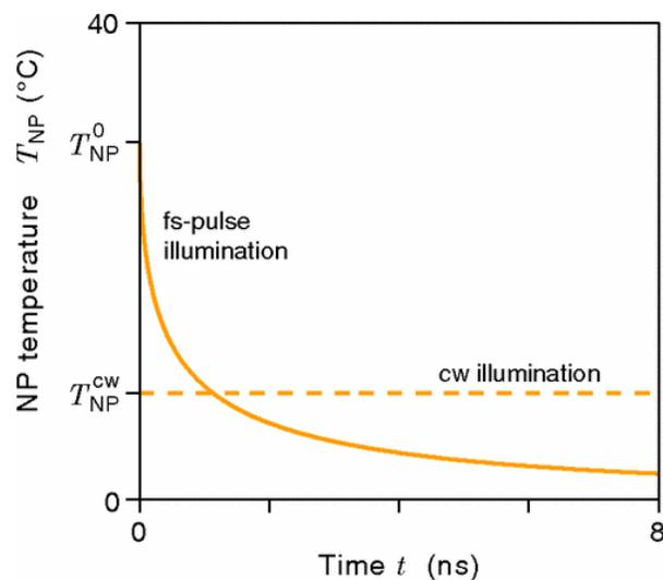
Figure 5-2. Evolution of the temperature of a nanoparticle with  $r = 50$  nm under pulsed light (solid line) and CW light (dashed line).<sup>11</sup>
