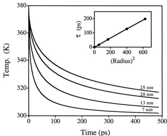
Figure 1-4: Calculated thermal responses of various sized nanoparticles.<sup>53</sup> From top to bottom, the different traces correspond to particles with radii of 25, 20, 13, and 7 nm. The inset shows the characteristic time constant for energy dissipation ( $\tau$ ) plotted versus the square of the radius.<sup>49</sup>
