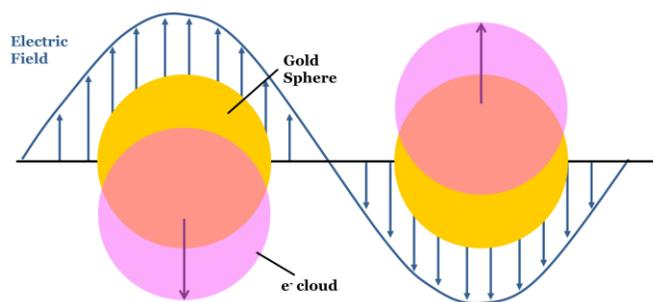
Figure 1-1: The production of a surface plasmon at the nanoparticle surface.
