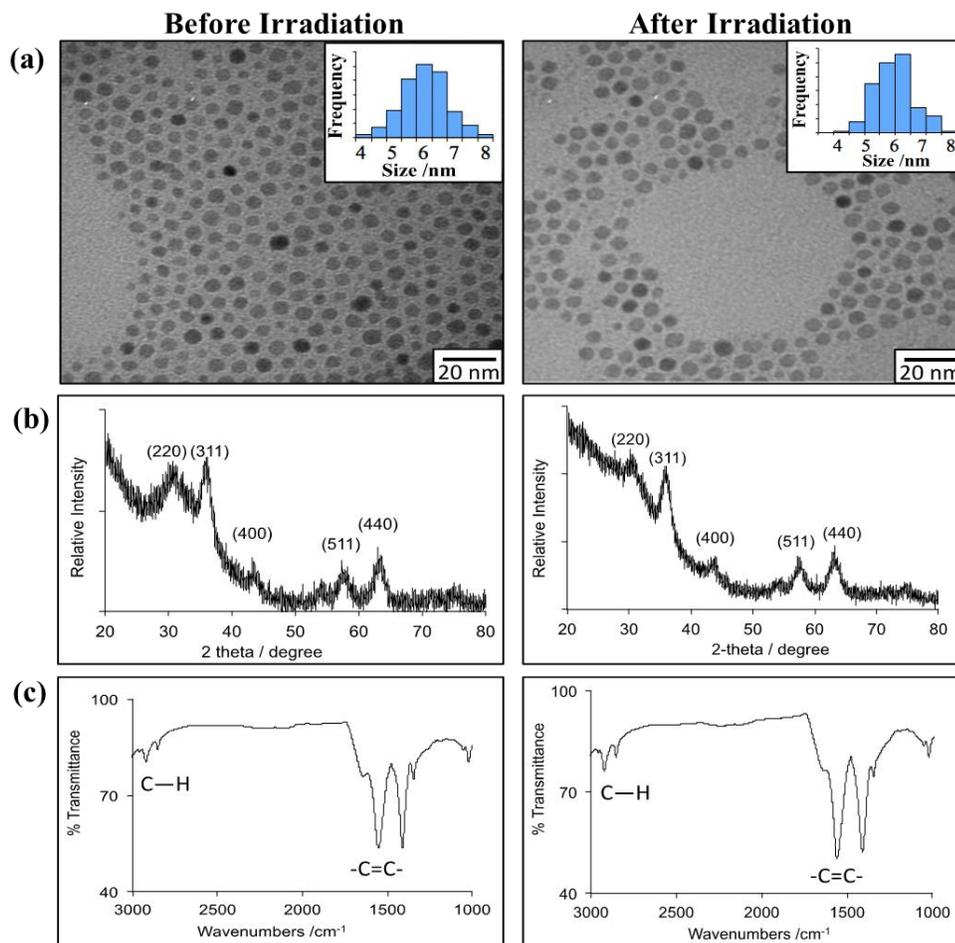
Figure 4-3. (a) TEM images, (b) XRD, and (c) IR spectra of MNPs before and after irradiation.<sup>22</sup>
