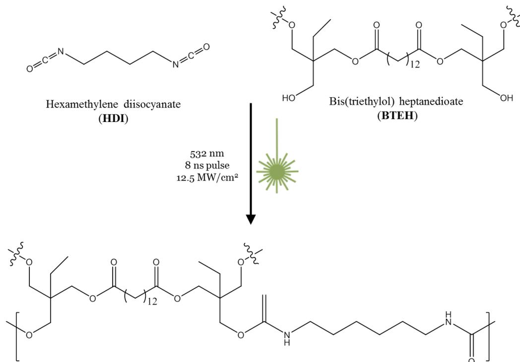
**Scheme 3-1.** Urethane formation reaction between hexamethylene diisocyanate (HDI) and diester polyol poly-bis(triethylol) heptanedioate (BTEH).
