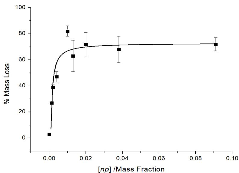
Figure 2-3. Change in the % mass loss versus mass fraction (concentration) of gold nanoparticles. Equation 1 is fit to this data (black curve).<sup>22</sup>
