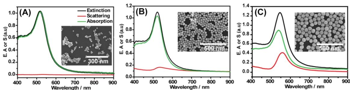
Figure 1-3: Extracted absorption and scattering spectra for gold nanoparticles of diameters a) 16.5 nm, b) 41 nm, and c) 72 nm.<sup>27</sup>
