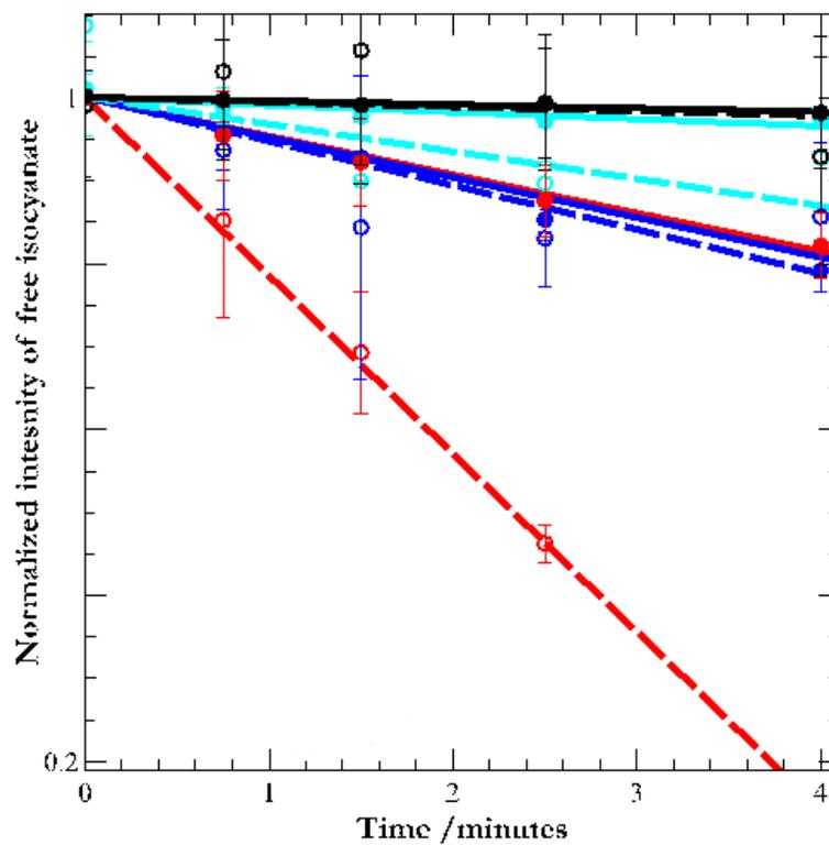
Figure 3-2. Kinetic traces following the disappearance of the isocyanate band (2274 cm<sup>-1</sup>)
