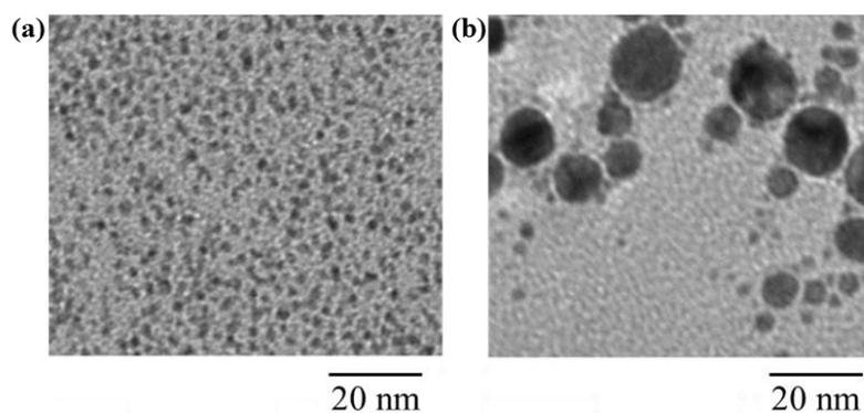
Figure 4-1. TEM of the PPC films containing AuNPs (a) before and (b) after irradiation.<sup>2</sup>
