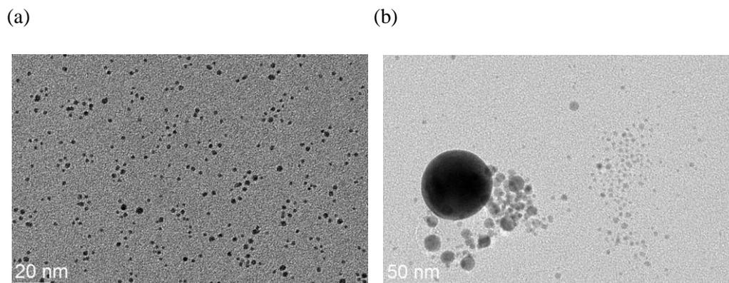
**Figure 3A-2.** TEM of AuNPs (a) before and (b) after irradiation.
