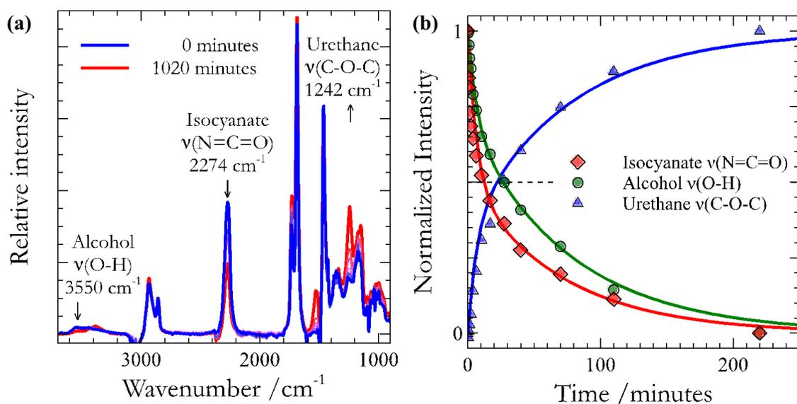
Figure 3-1. The reaction between HDI and BTEH to form polyurethane followed using (a) infrared spectroscopy. In particular, we observe the loss of bands associated with the isocyanate ( $2274\text{ cm}^{-1}$ ) and alcohol ( $3550\text{ cm}^{-1}$ ) moieties, and the appearance of the C-O-C mode ( $1242\text{ cm}^{-1}$ ) associated with the urethane. (b) The kinetics associated with these changes indicate direct conversion to urethane.
