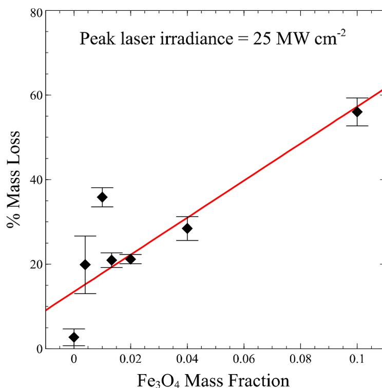
Figure 4-2 PPC films containing MNPs were irradiated and their % mass loss was plotted vs concentration of MNPs.<sup>22</sup>
