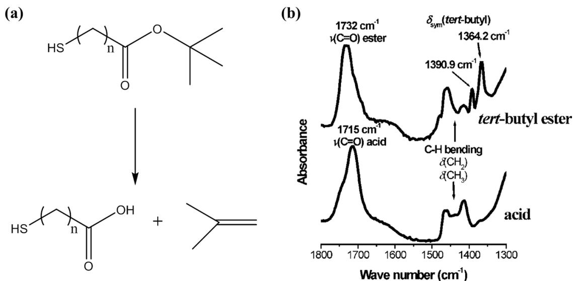
Figure 5-1. (a) Ester cleavage can be accomplished at high temperatures, and the progress of this reaction can be monitored by (b) following changes in the IR spectrum.<sup>10</sup>
