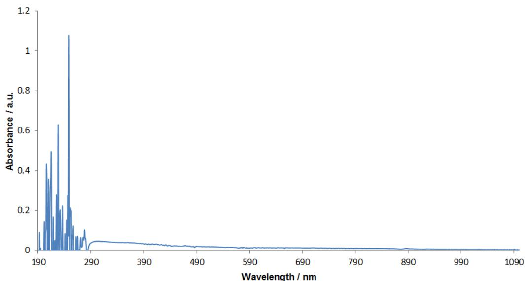
**Figure 3A-3.** UV-Vis spectrum of 0.07% w/v solution of DBTDL in toluene.
