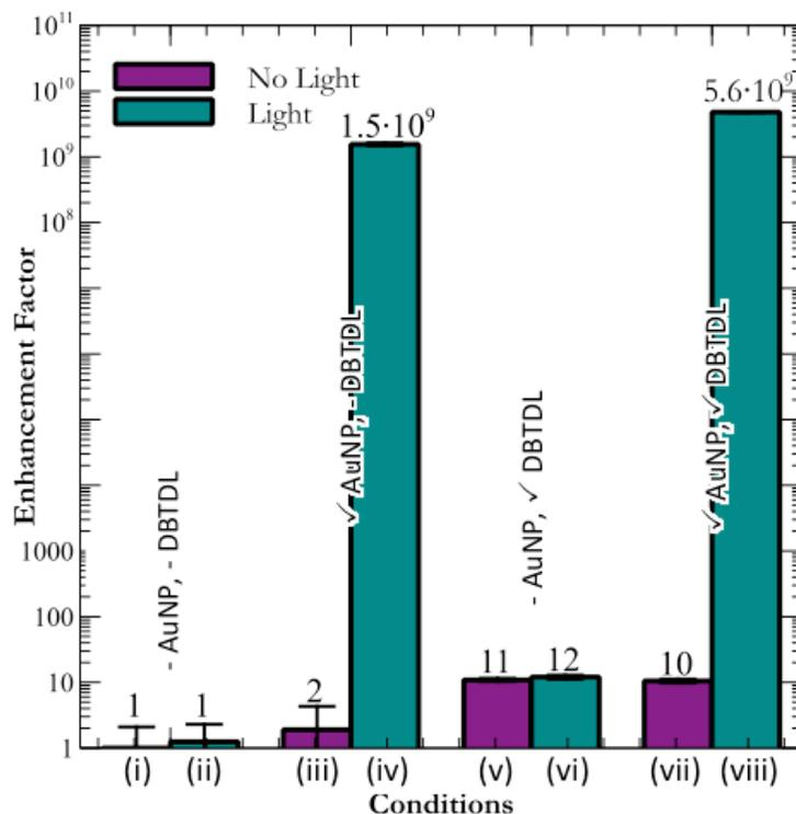
Figure 3-4. The relative rate of reaction (with respect to pure polymer) for all eight conditions calculated using the total irradiation time of 20  $\mu$ s for samples experiencing photothermal heating.
