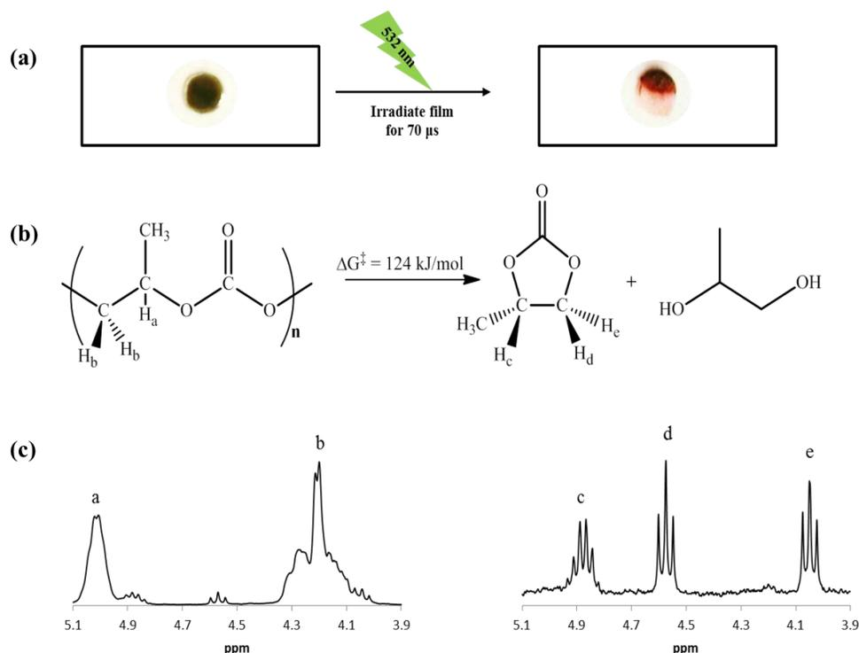
Figure 2-1. (a) The course of a general experiment. (b) Chemical equation for the depolymerization of polypropylene carbonate (PPC) by chain unzipping. (c)  $^1\text{H}$  NMR of the polymer blend before (left) and after (right) irradiation.<sup>22</sup>
