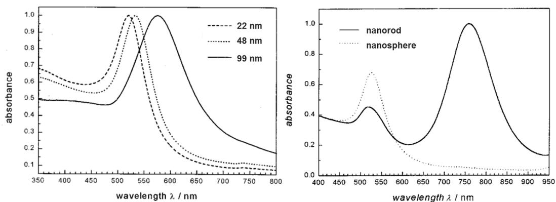
Figure 1-2: UV-Vis spectra of various gold nanoparticles, showing how a) size and b) shape of gold nanoparticles affect the SPR.<sup>12,22</sup>
