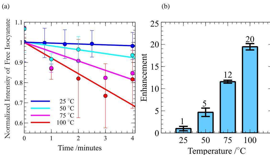
**Figure 3A-4.** (a) Early time kinetics of polyurethane film formation over time at various temperatures. (b) The enhancement of the kinetics at these temperatures, relative to the room temperature rate.
