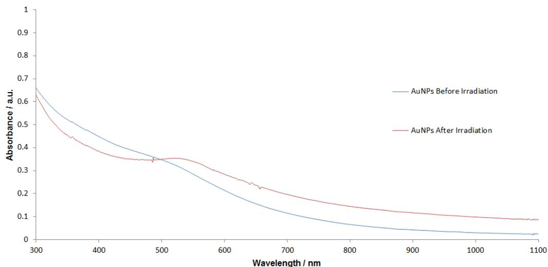
**Figure 3A-1.** UV-Vis spectrum of AuNPs before and after irradiation
