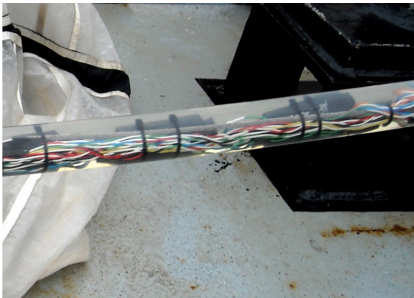
Figure 2.2: Close up of oil filled towed array used for marine biology research (Gogan, 2014)
