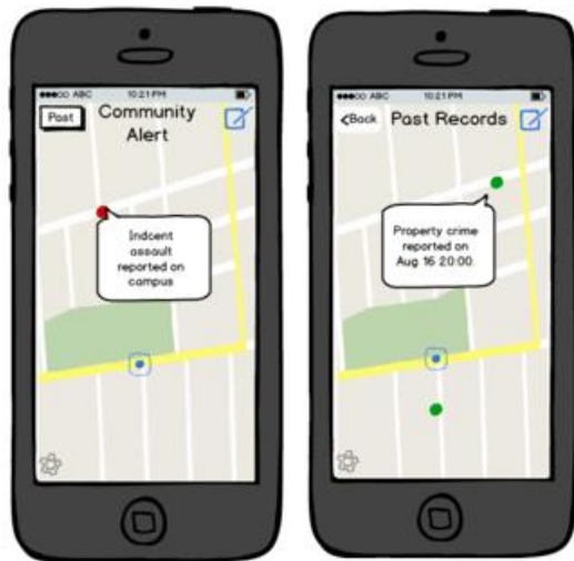
Figure 3-5. High fidelity prototypes; Left: Landing page of app showing the emergency (red dot) with respect to user’s position (blue dot); Right: Page showing past incidents (green dots)
