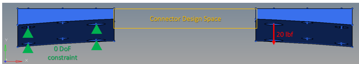
Figure 4-24. Connector optimization and analysis load case 2
