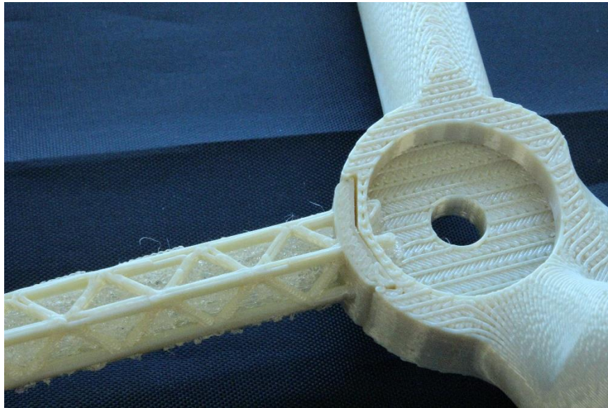
Figure 4-32. Dovetail connection design (credit Corey Dickman)
