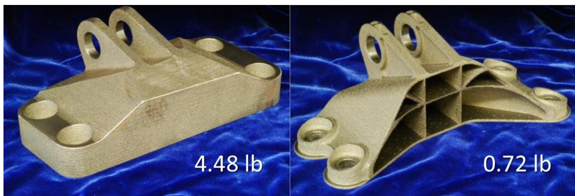
Figure 1-5. GE Bracket Challenge original part (left) and winner (right) [1]
