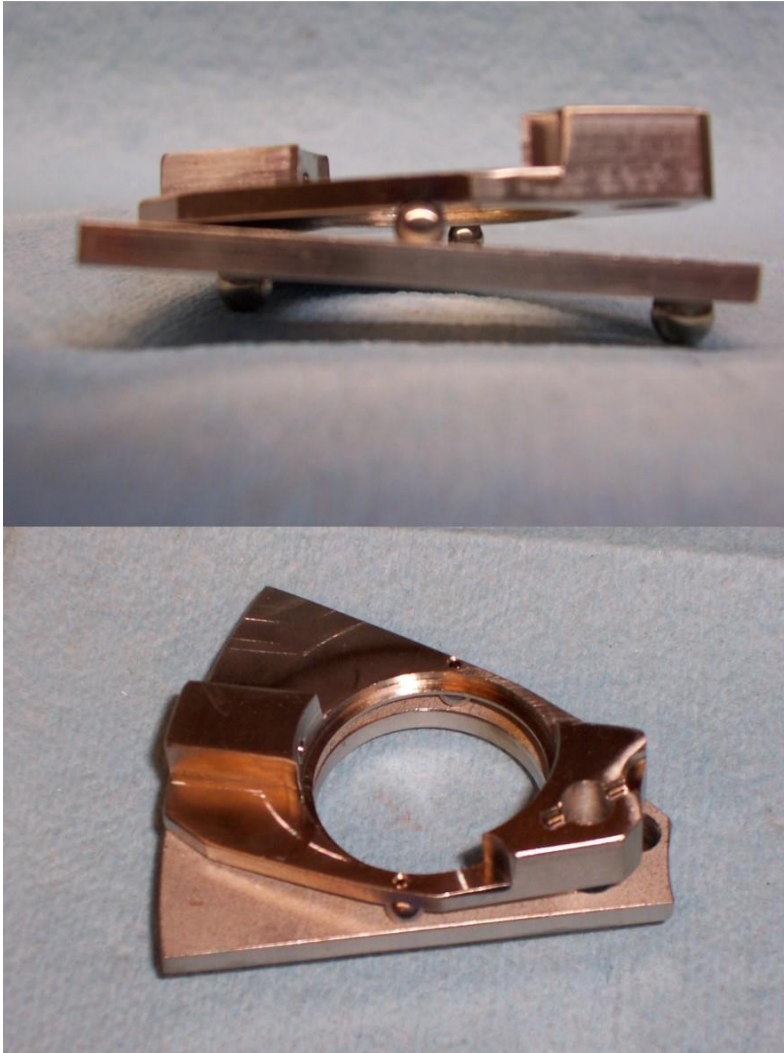
Figure A.5. Photographs of the wedge/sub-wedge assembly simply to show how the pieces are coupled.
