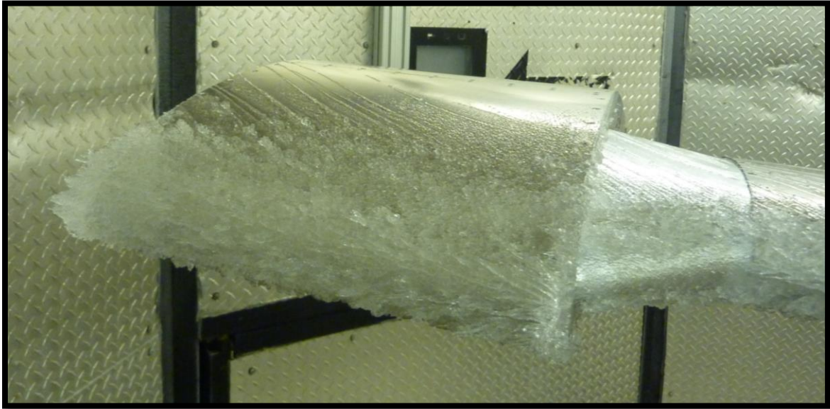
Figure 3-7. Glaze ice - LWC: 0.45 \text{ g/m}^3 , MVD: 18\mu\text{m} , T: -3^\circ \text{C} , Time: 15 min.
