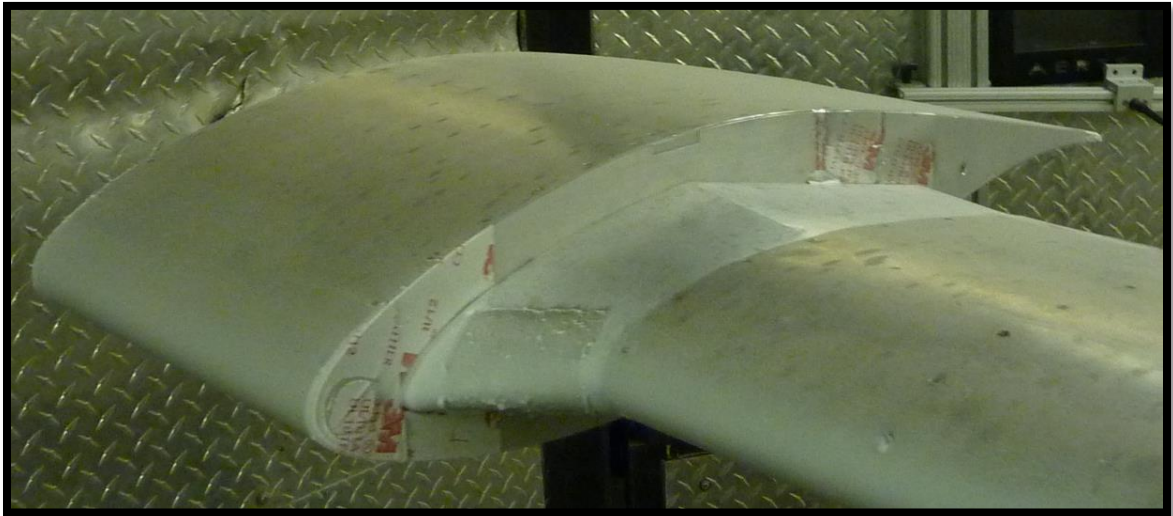
Figure 3-6. Rime Ice - LWC: 0.21 \text{g}/\text{m}^3 , MVD: 20 \mu\text{m} , T: -21 ^{\circ}\text{C} , Time: 2 min.
