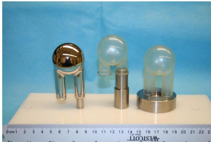
**Figure 3-1: The steel mandrel is shown to the left, the sac used in the PVAD with the heat-formed ports is shown in the middle and the sac after removal from the mandrel is shown on the right.**
