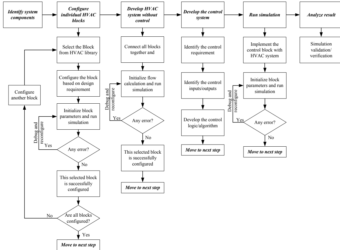
Figure 5-2 Flow chart of developing the Simulink model simulation.
