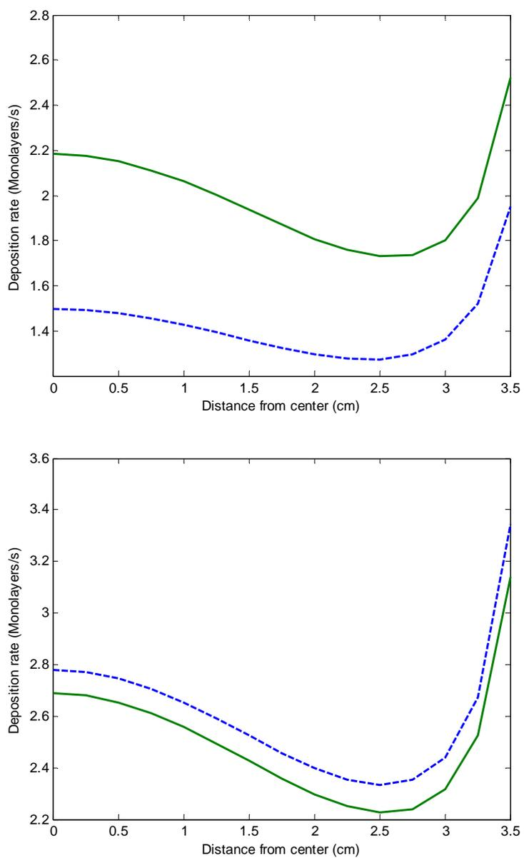
Figure 5-3: Uniformity profiles at starting conditions (dashed) and optimal conditions (solid) for Ga (top) and Al (bottom) for annealing time only formulation using Nelder-Mead
