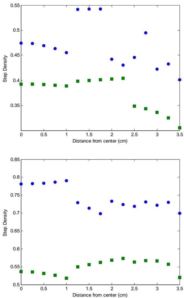
Figure 5-4: Step density profiles at starting conditions (circles) and optimal conditions (squares) for Al over Ga (top) and Ga over Al (bottom) for annealing time only formulation using Nelder-Mead
