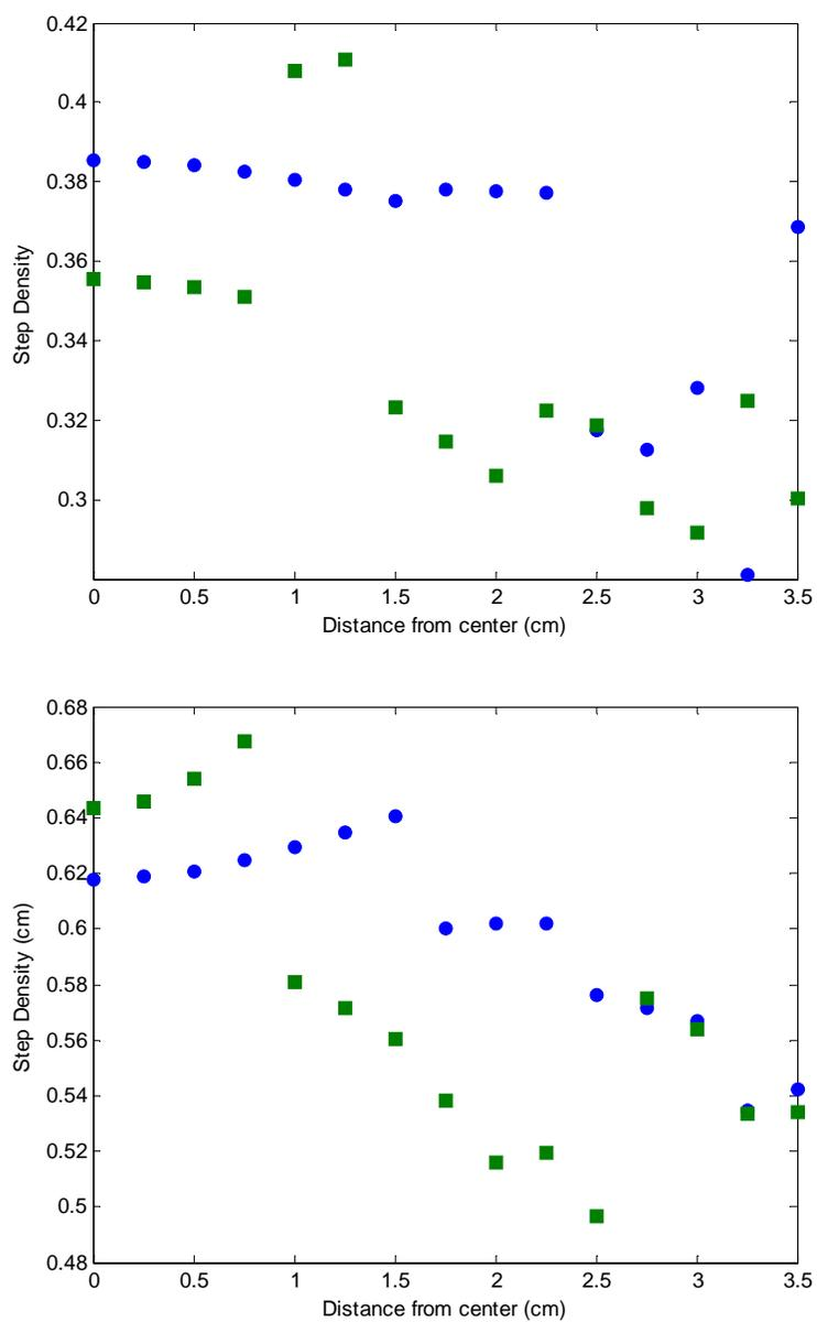
Figure 5-6: Step density profiles at starting conditions (circles) and optimal conditions (squares) for Al over Ga (top) and Ga over Al (bottom) for “off-time” formulation using Nelder-Mead
