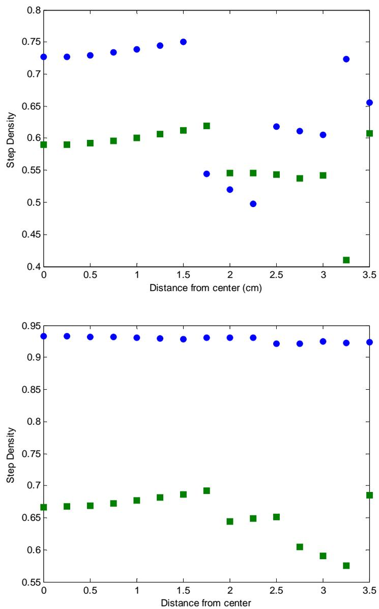
Figure 5-10: Step density profiles at starting conditions (circles) and optimal conditions (squares) for Al over Ga (top) and Ga over Al (bottom) for annealing time only formulation using Hooke-Jeeves
