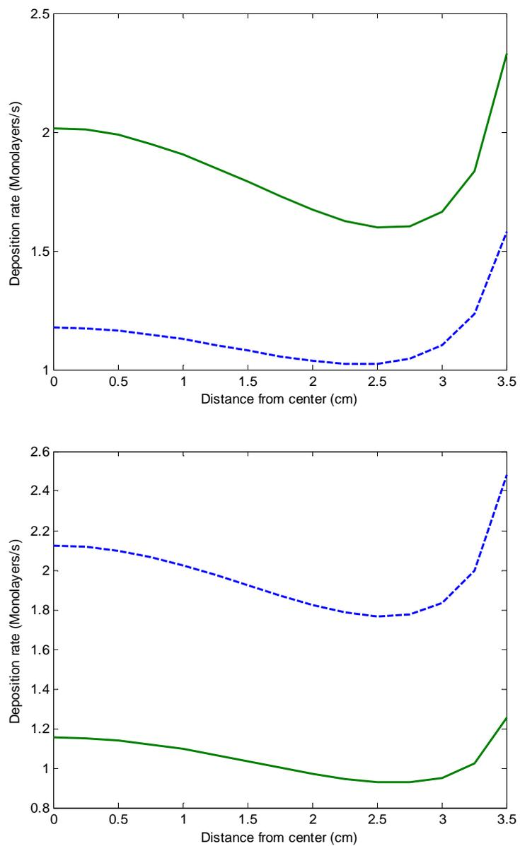
Figure 5-9: Uniformity profiles at starting conditions (dashed) and optimal conditions (solid) for Ga (top) and Al (bottom) for annealing time only formulation using Hooke-Jeeves
