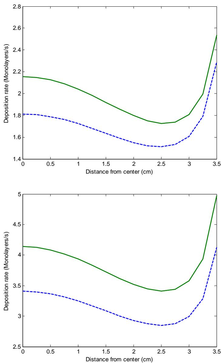
Figure 5-5: Uniformity profiles at starting conditions (dashed) and optimal conditions (solid) for Ga (top) and Al (bottom) for “off-time” formulation using Nelder-Mead
