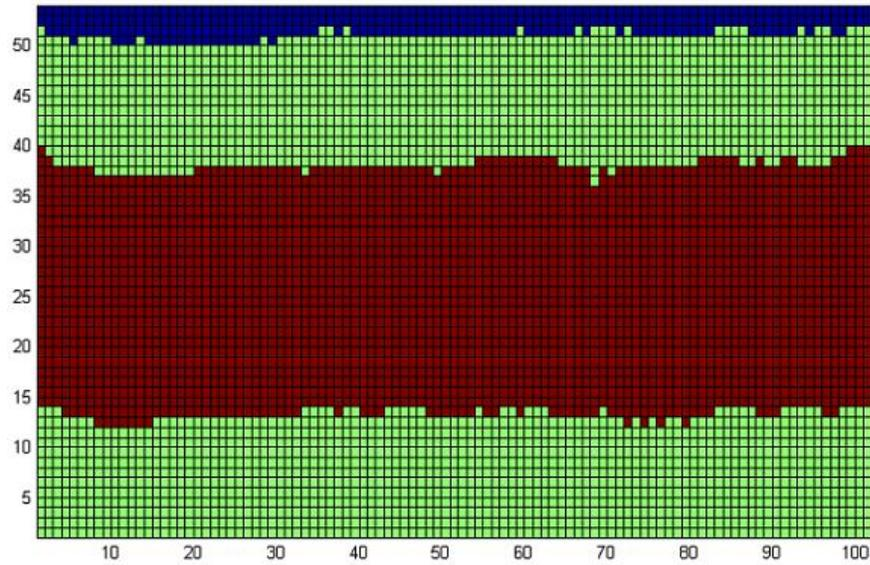
Figure 5-7: Cross-section of wafer at “optimal” conditions, wafer center, for annealing time only formulation using Nelder-Mead
