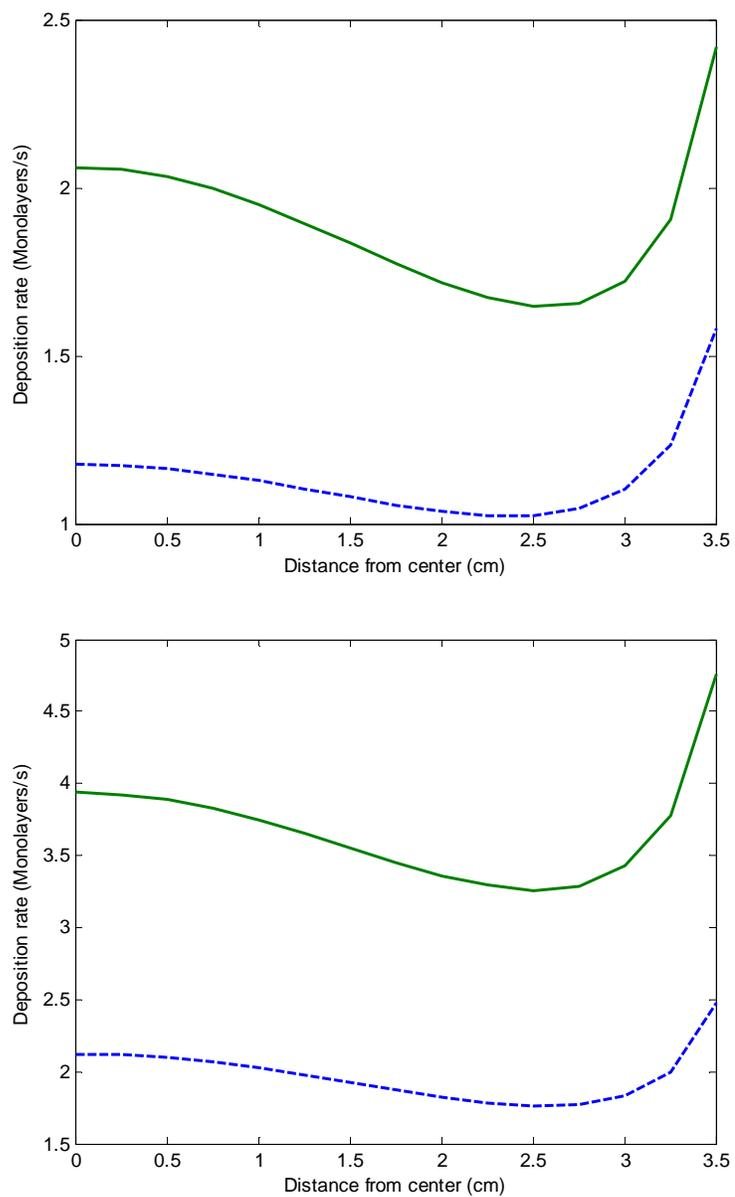
Figure 5-11: Uniformity profiles at starting conditions (dashed) and optimal conditions (solid) for Ga (top) and Al (bottom) for “off-time” formulation using Hooke-Jeeves
