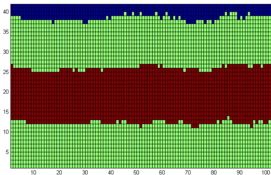
Figure 5-13: Cross-section of wafer at “optimal” conditions, wafer center, for annealing time only formulation using Hooke-Jeeves
