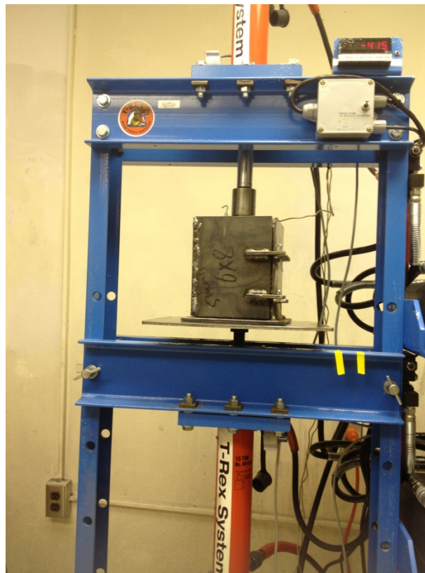
Figure 4. 7. The T-Rex machine compressing biomass.
