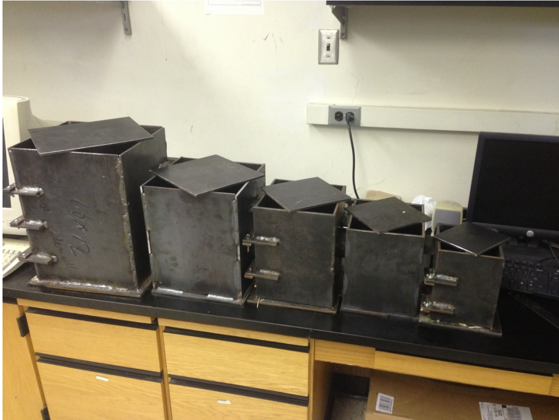
Figure 4. 4. The chambers of different size (left to right: V, IV, III, II, I).
