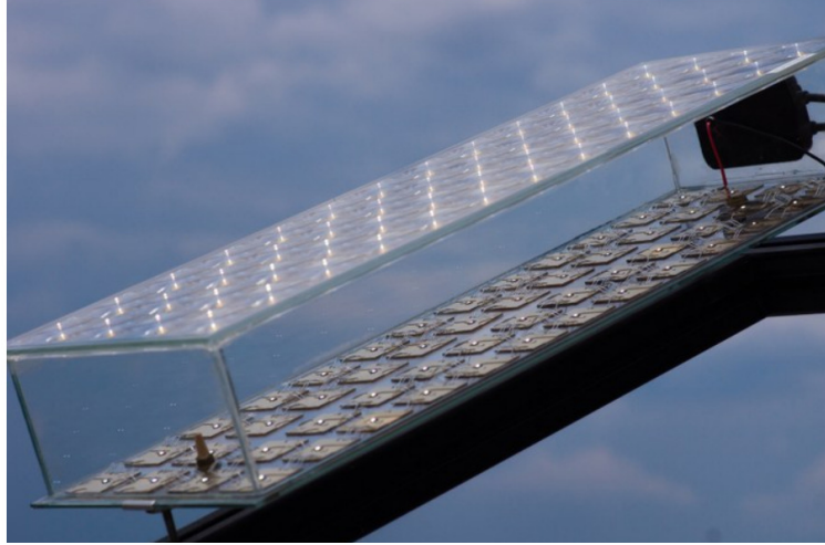
Figure 1.2. Soitec’s FLATCON module which utilizes only a single Fresnel lens to couple light to multijunction PVs. This particular design set a world record for module efficiency at 36.7% in July of 2014.
