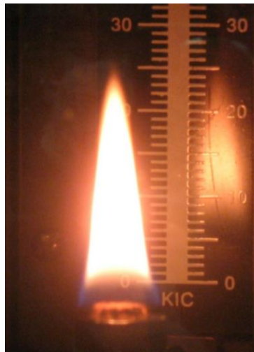
Figure 5 Photograph taken of an iso-octane/toluene diffusion flame at the smoke point.
