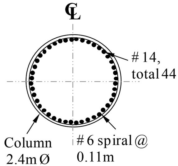
Figure 3-1. (c) Column cross-section
