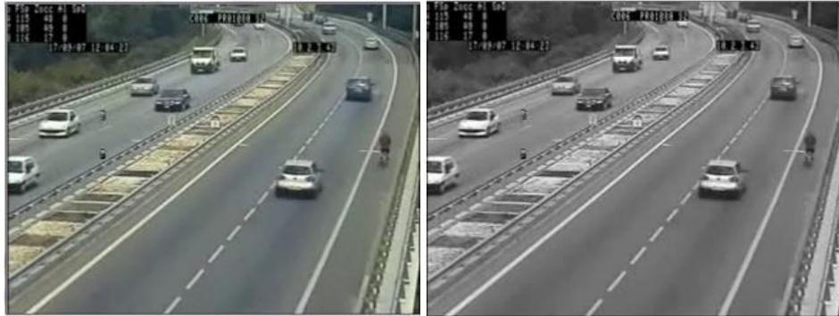
Figure 3-2: Illustration of Step 1. Original frame in BGR color space (left), Frame after processing in Step 1 in Gray color space (right)
