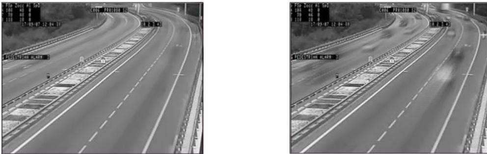
Figure 3-4: Extracted background when  $\alpha$  equals 0.01 (left) and when  $\alpha$  equals 0.1(right)
