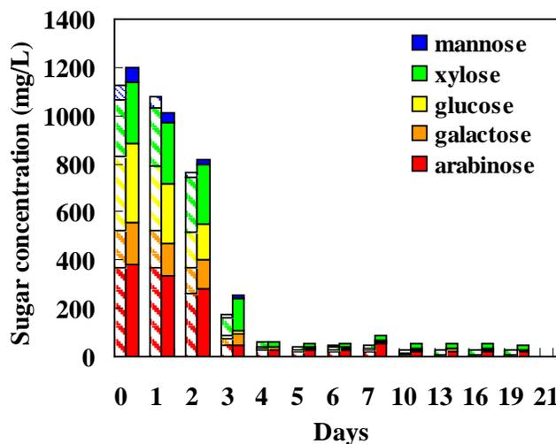
Figure 4-18. Sugar concentration change with time in integrated digestion and control for Batch 2 data. The column with strips data was from integrated digestion, and the solid column data was from control. The colors presented in the legend for individual sugars applied to both integrated digestion and control data.
