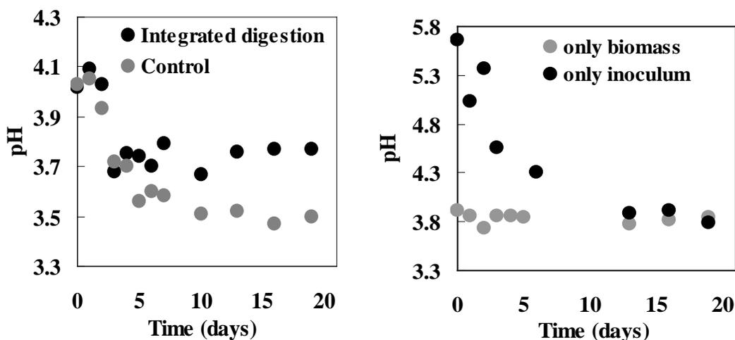
Figure 4-19. pH of integrated digestion, control, only biomass with the same solid loading rate without inoculation, and only inoculum with the same solid loading rate without biomass.
