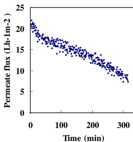
Figure 4-12. Permeate flux change with time during a single filtration event from Batch 1. Filtration condition: 5 bar, pH 3.49. Feed solution is the digestion liquor from day 15 containing 2.8 g/L lactic, 0.05 g/L formic, 0.46 g/L acetic, 2.7 g/L propionic, 2.2 g/L butyric and 23.3g/L hexanoic acid.
