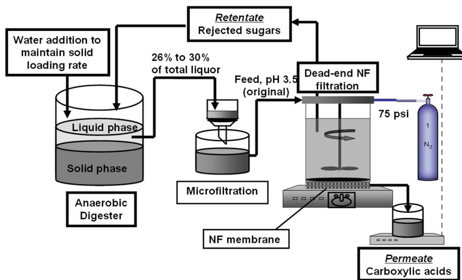
Figure 3-3. Flow chart of Phase 3 integrated digestion and separation.
