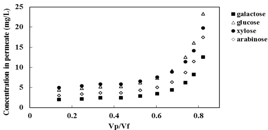
Figure 4-15. Sugar concentration changes in the permeate during filtration on day 10. Filtration condition: 5 bar, pH 3.49. The day 10 digestion liquor contained 29.7 mg/L arabinose, 26.8 mg/L galactose, 42.8 mg/L glucose, 20.9 mg/L xylose.
