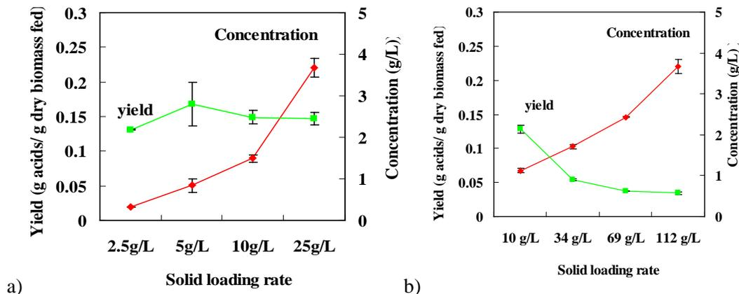
Figure 4-1. Total acid yield and concentration for two different ranges of solid loading rates at day 10. a). Low range: 2.5g/L to 25 g/L; b). high range: 10g/L to 112 g/L. Solid loading rate unit indicated g dry biomass/L.
