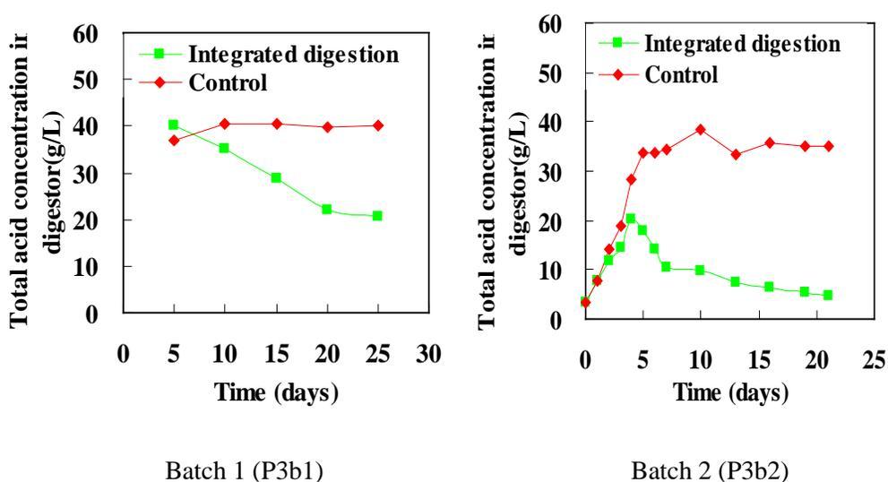
Figure 4-16. Total acid concentration changes with time in the integrated digestion and separation system. The concentration of reported for batch 1 (P3b1) is the concentration measured every time before acid removal and that from batch 2 (P3b2) is the concentration measured after acid removal.
