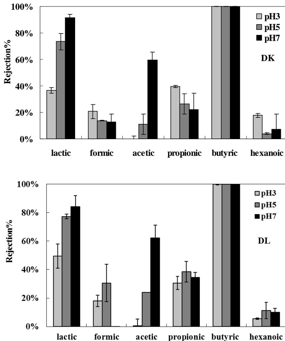
Figure 4-5. Carboxylic acid rejection at three different pH values, a pressure of 8 bar, and a temperature of 25 °C using two NF membranes, DK and DL. Error bars of carboxylic acid rejection indicate standard error for duplicate sets of filtration experiments.
