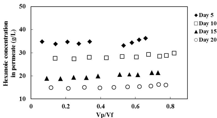
Figure 4-14. Hexanoic acid concentration change in the permeate during filtration on days 5, 10, 15 and 20.
