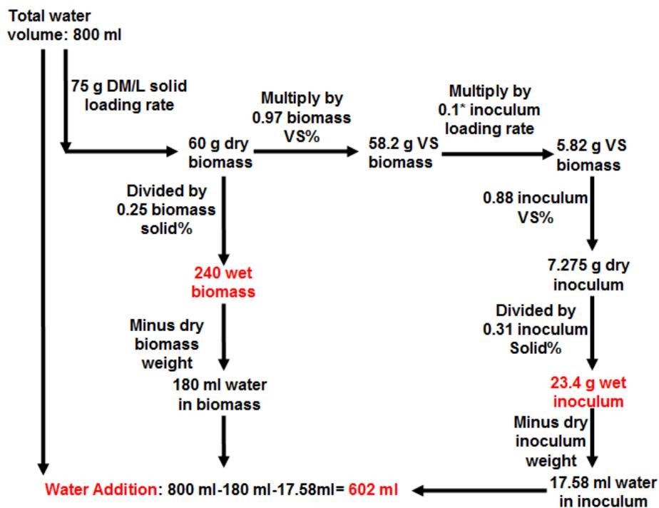
Figure 3-1. Flow chart of an example of determining wet biomass and inoculum quantity in prior to willow wood digestion. \* Inoculum loading rate is in g VS inoculum/ g VS biomass. Solid% indicates dry biomass fraction, and VS% indicates volatile solids fraction on dry biomass basis.
