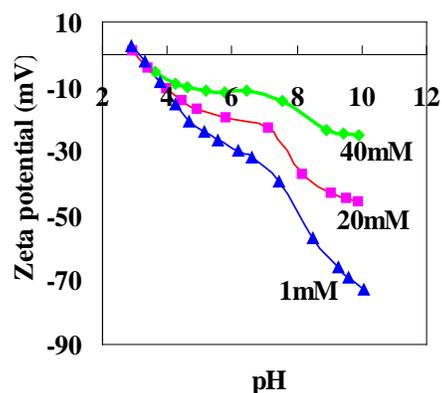
Figure 5-1. Zeta potential of DL membrane under 3-10 pH conditions with 1mM, 20 mM and 40mM NaCl solution as background electrolyte.
