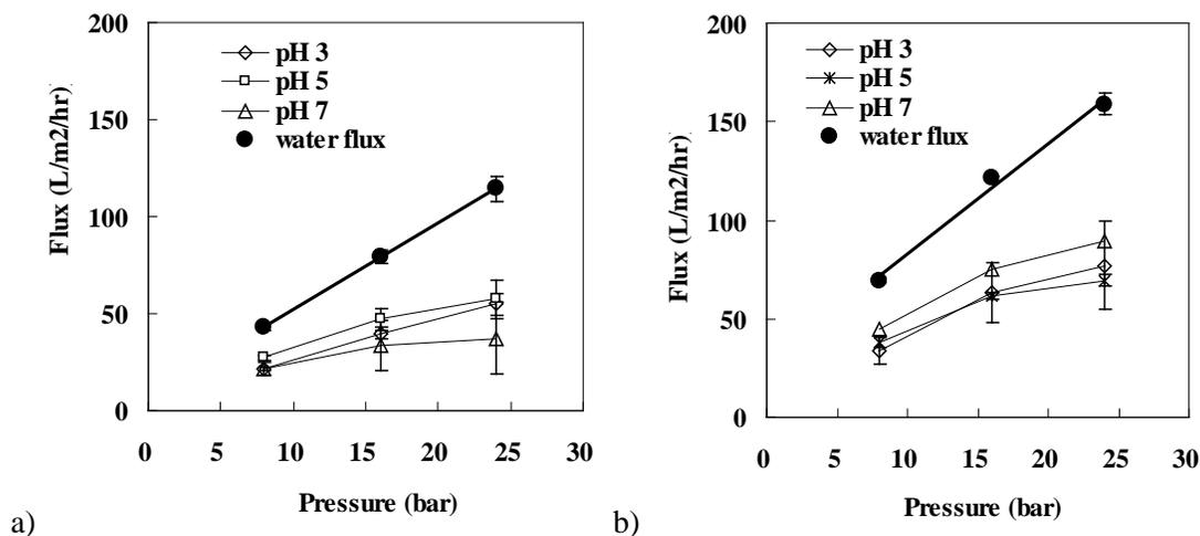
Figure 4-9. Sample flux is reported as a function of applied pressure. The control is pure water flux without pH adjustment, while digestion liquor sample flux was tested at three different pH values, all at 25°C. a) DK membrane, b) DL membrane. Error bars for the sample flux indicate the standard error for duplicate filtration experiments. Error bars of pure water flux indicate the standard error for six replicate experiments.
