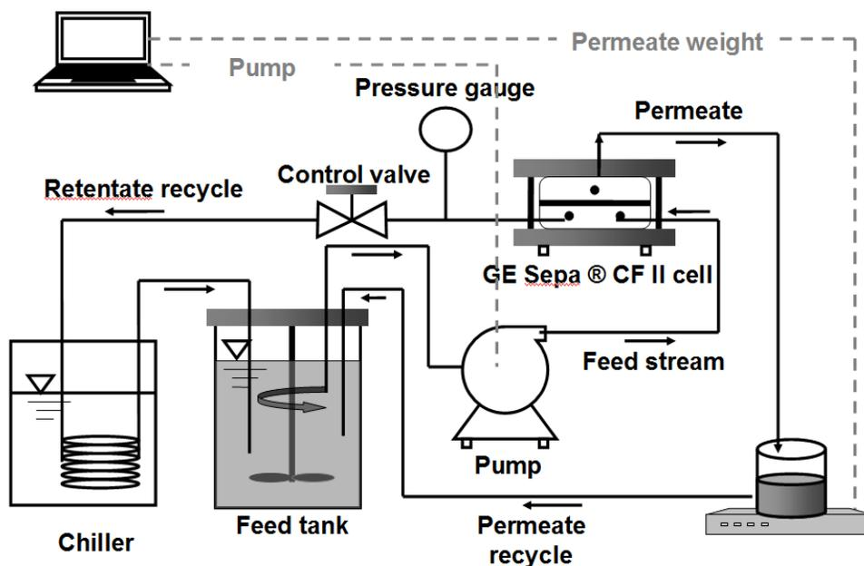
Figure 3-2. Schematic diagram of cross-flow filtration system in constant pressure operation mode.
