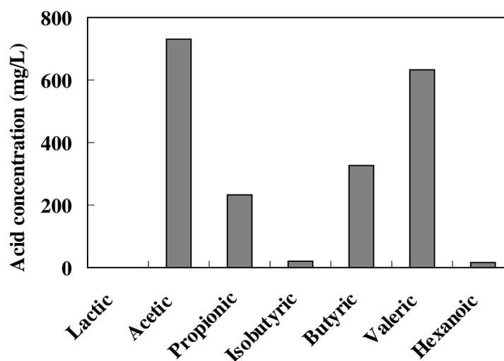
Figure A-3. Carboxylic acid concentration in 42 day old digestion liquor of pretreated switchgrass with 10 g DM/L solid loading rate.
