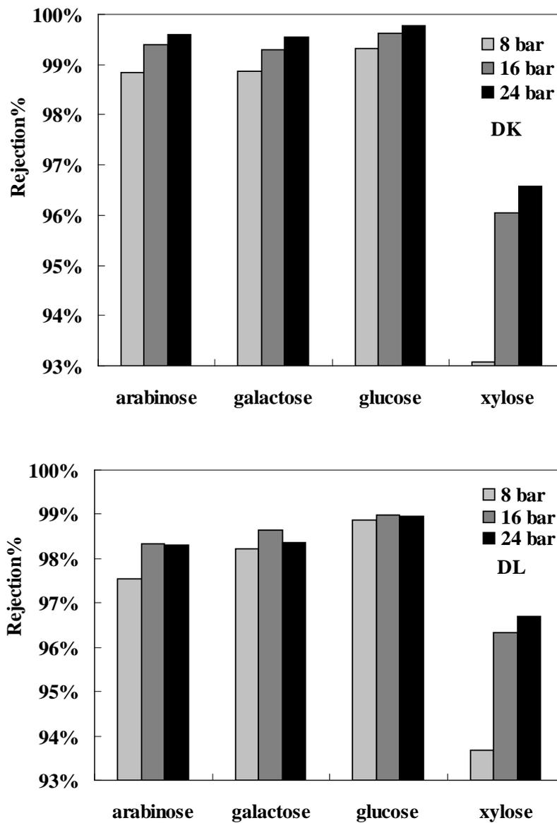
Figure 4-11. Sugar rejection at three different pressures at pH 3 and 25°C for two NF membranes, DK and DL. Arabinose, galactose and glucose data were from one single set of experiments. Xylose data was from duplicate experiments. Data with standard error of the xylose are presented below in the order of DK first with three pressures from 6 to 8 bars, and then DL with same pressure order: 93.1%±0.3%, 96.1%±0.4%, 96.6%±0.4%, 93.7%±1.8%, 96.3%±1.7%, 96.7±2.0%.
