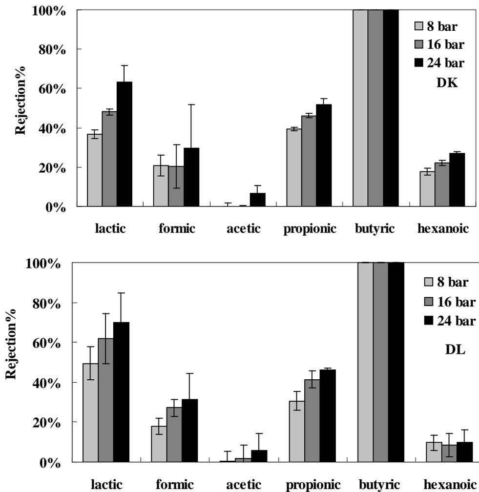
Figure 4-10. Carboxylic acid rejection at three different pressures at pH 3 and 25 °C for two NF membranes, DK and DL. Error bars for carboxylic acid rejection indicate standard error for duplicate sets of filtration experiments.
