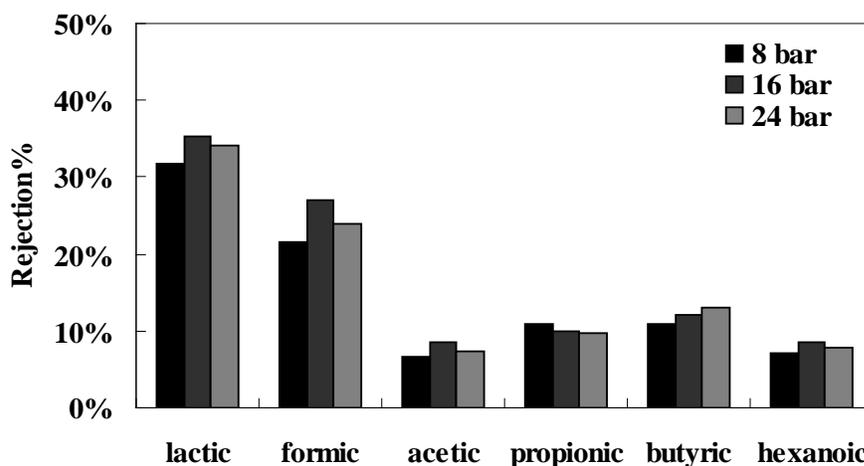
Figure 4-6. Carboxylic acid rejection using a synthetic model solution with initial pH 2.4, at three different pressures, and a temperature of 25 °C, using DL membrane. Data was from one set of filtration experiment.
