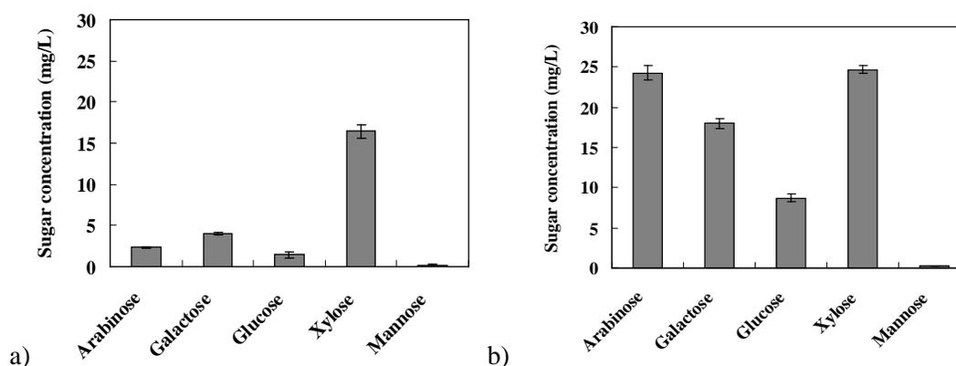
Figure 4-4. Monosaccharide concentration in 10 day old digestion liquor of pretreated a) Willow 1 and b) Willow 2. The digestion was with 75 g DM/L solids loading rate.
