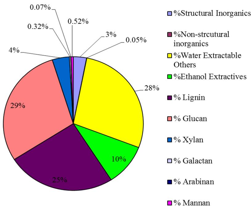
Figure A-2. Chemical composition of hot water pretreated willow wood. Pretreatment condition: 190°C, 5 minutes on AdvanceBio hydrolyzer.
