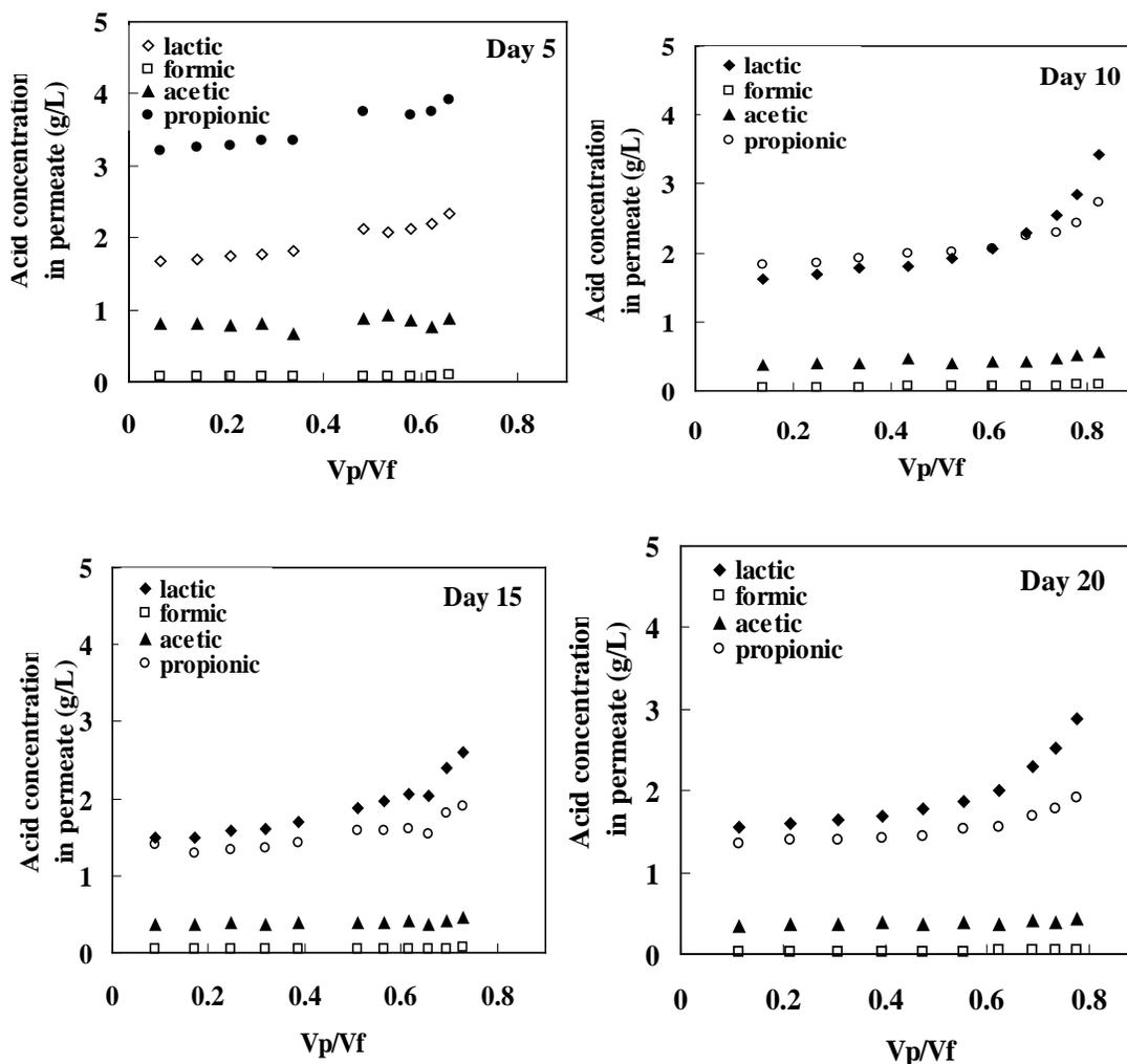
Figure 4-13. Changes in lactic, formic acetic and propionic acid concentrations in the permeate during filtration on days 5, 10, 15 and 20.  $V_p/V_f$  represents the ratio of the volumes of permeate and feed.
