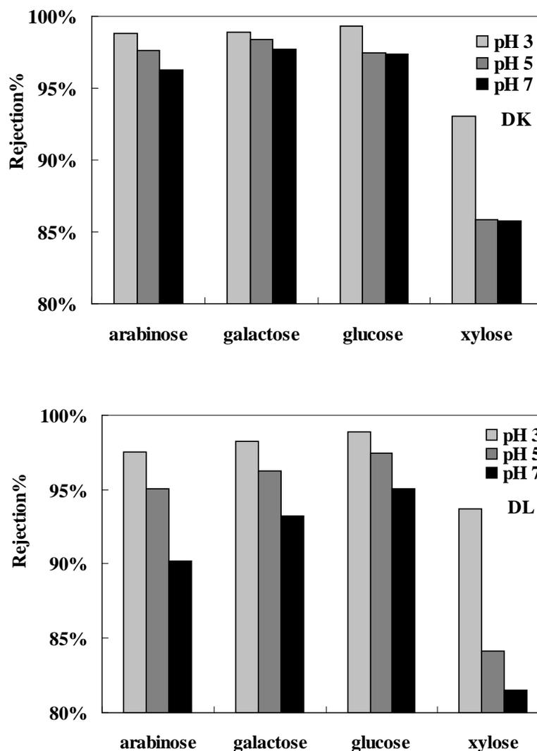
Figure 4-8. Sugar rejection at three different pH values at 8 bar, 25°C with two NF membranes. Arabinose, galactose and glucose data were from one single set of experiments. Xylose data was from duplicate experiments. Data with standard error of the xylose are presented below in the order of DK first with three pH values from pH 3 to 7, and then DL with same pH order: 93.1%±0.3%, 85.5%±3.8%, 85.8%±1.0%, 93.7%±1.7%, 84.1%±1.6%, 81.5%±10.1%,
