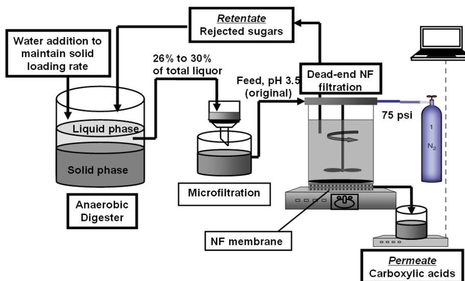
Figure 3-4. Flow chart of Phase 3 integrated digestion and separation.
