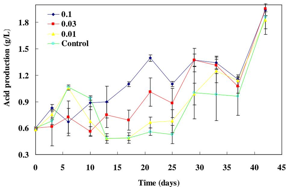
Figure 4-2. Acid concentration with different inoculum loading rates (g VS inoculum/ g VS biomass). The control was acidogenic digestion without inoculation. All trials used a 10 g DM/L solids loading rate. Error bars are the standard error of triplicate experiments.
