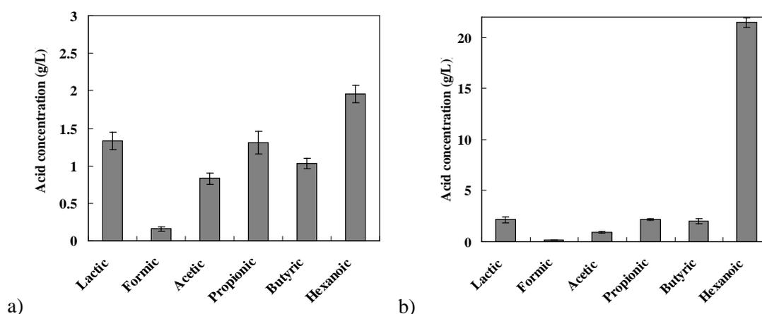
Figure 4-3. Carboxylic acid concentration in 10 day old digestion liquor of pretreated a) Willow 1 and b) Willow 2. The digestion was with 75 g DM/L solids loading rate.
