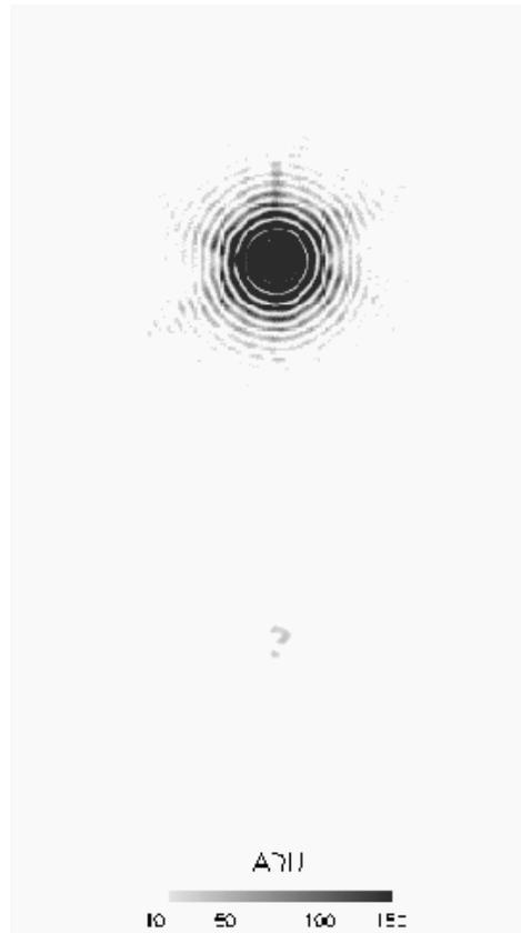
Fig. 5.10 (top) 10 second image of the laser point source without the mask in place. (bottom) Image with same intensity stretch with the mask in place. The peak pixel value of the bottom image is  $2.8 \times 10^5$  ADU.
